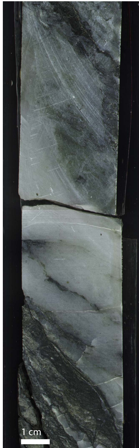
Figure F29. Example of large patch (or vein?) of anhydrite that consumes the width of the core (interval 108Z-4, 9–30 cm).
