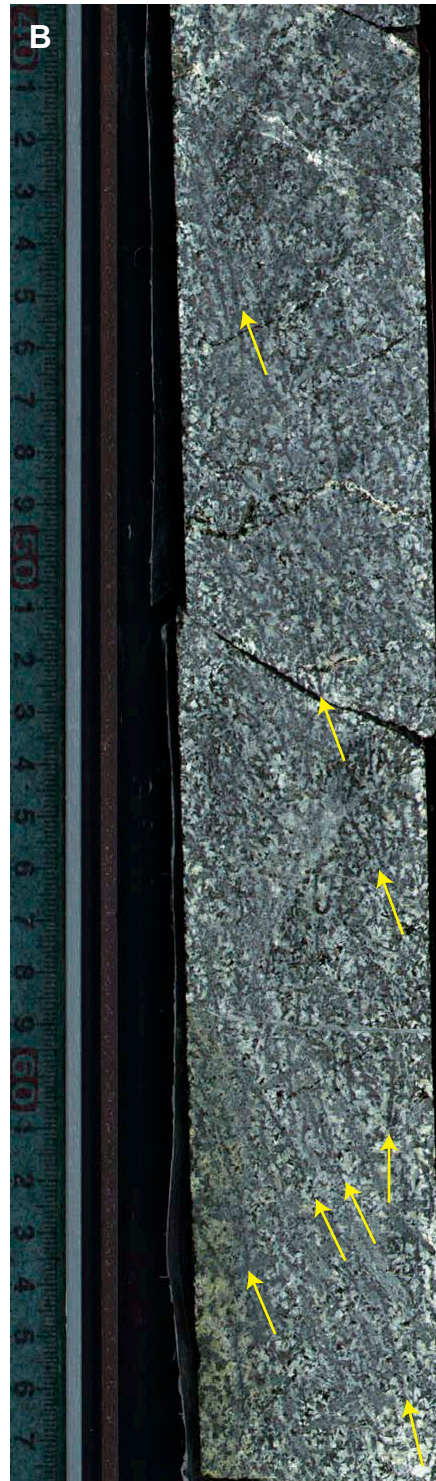
Figure F9. Typical oxide gabbros. A. Textural and grain size variations. B. Dendritic amphibole (yellow arrows), probably of rapid-growth clinopyroxene/hornblende origin.
