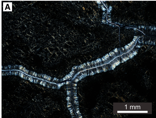
Figure F29. Selected examples of typical veins in dunite and harzburgite lithologies, Hole BA4A. A. Edge-shaped aggregates of two serpentine phases. B. Microcrystalline serpentine in the middle of two-phase serpentine vein. C. Serpentine veins with overlapping connectivity cut through the magnetite-bearing serpentine veins. D. Composite serpentine veins with twin calcite in the middle. E. Colloform calcite with serpentine (Srp) islands in the middle. F. Radial needle-like aggregate of xonotlite.
