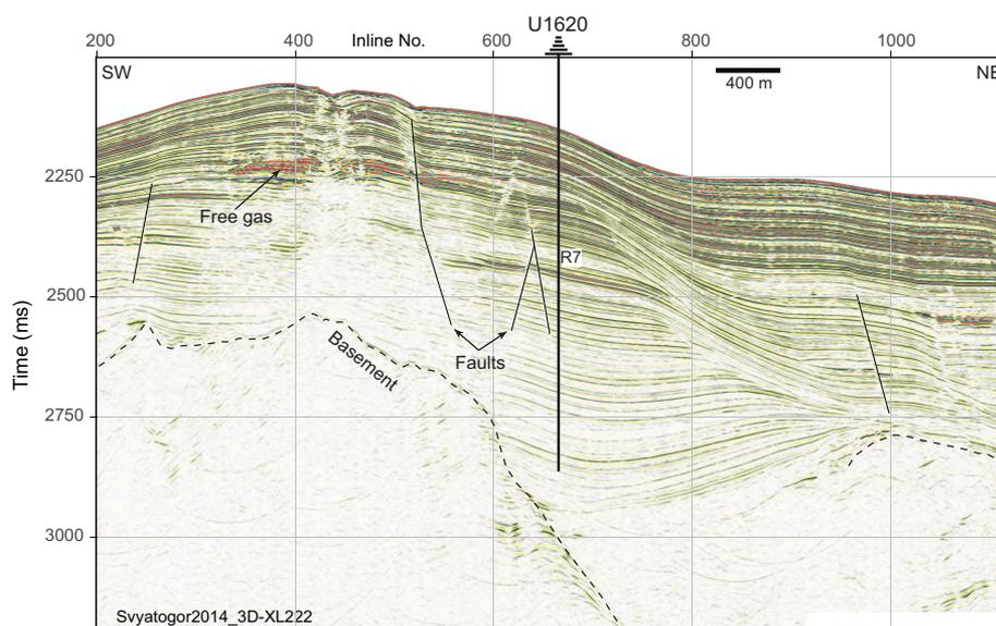
**Figure F14.** Seismic profile along southwest–northeast Seismic Line Svyatogor2014\_3D-XL222 showing the location of Site U1620 with interpreted Reflector R7 and the maximum penetration depth of 616 mbsf. Interpreted location of the underlying basement, multiple faults, and free gas are also shown.
