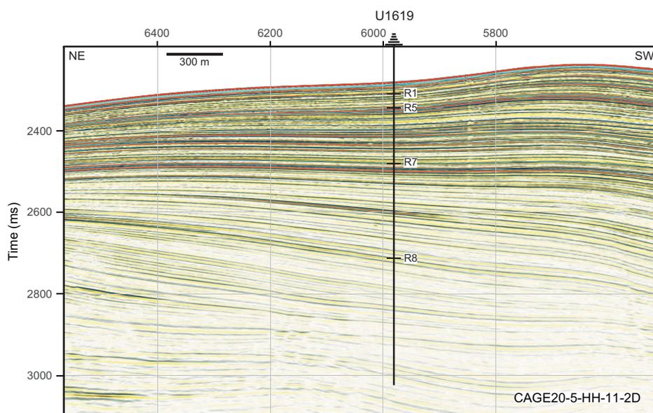
**Figure F13.** Seismic profile along northwest–southeast Seismic Line CAGE20-5-HH-11-2D showing the location of Site U1619 with interpreted Reflectors R1–R8 and the maximum penetration depth of 627.9 mbsf.
