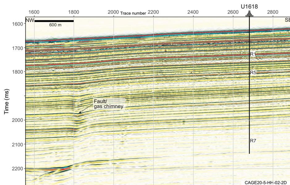
**Figure F6.** Seismic profile along northwest–southeast Seismic Line CAGE20-5-HH-02-2D showing the location of Site U1618 annotated with interpreted Reflectors R1, R5, and R7 and the maximum penetration depth of 414 mbsf. Interpreted locations of a fault and possible gas chimney are indicated.
