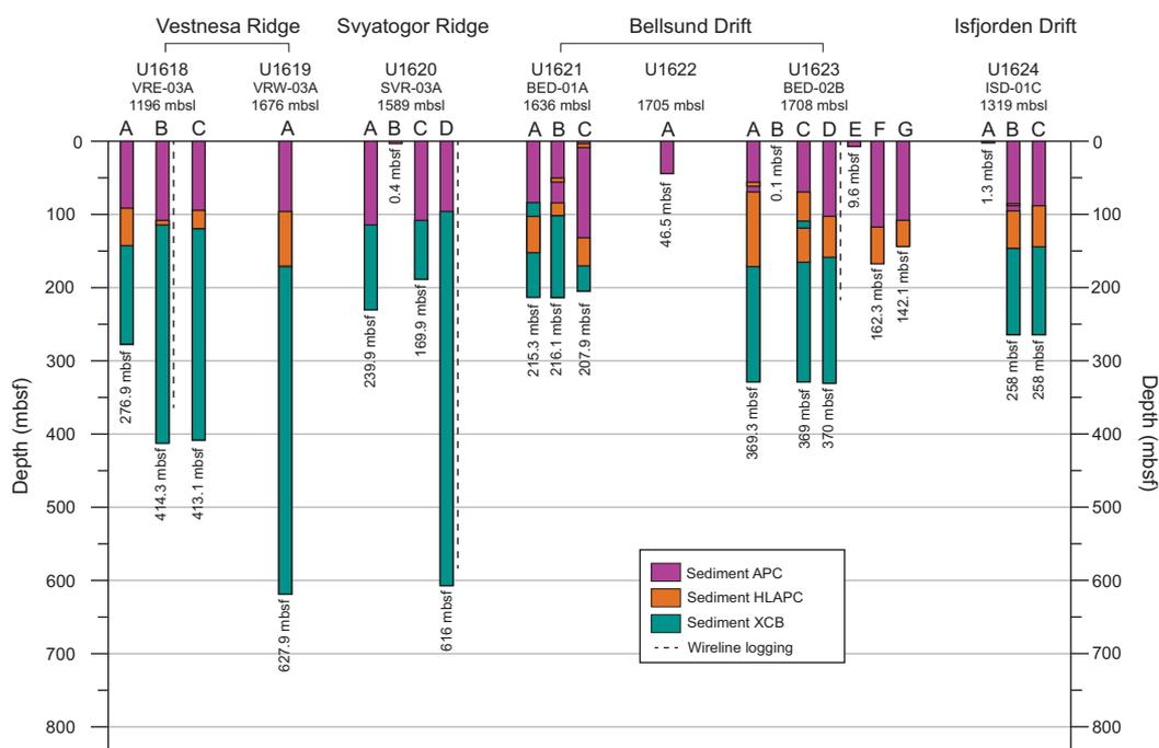
**Figure F5.** Drilling operations, Expedition 403. Sites and holes are organized (left to right) in order of operation, except for Holes U1623D–U1623G, which were drilled upon return to the site following operations at Site U1624.
