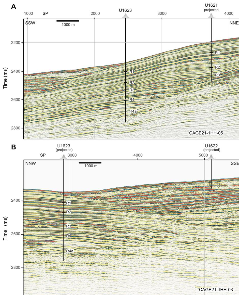
**Figure F15.** A. Seismic profile along northwest–southeast Seismic Line CAGE21-1-HH-05 showing the projected location of Site U1621 and the location of Site U1623 with interpreted Reflectors R1–R4a and the maximum penetration depth of 216 mbsf (Site U1621) and 370 mbsf (Site U1623). B. Seismic profile along northwest–southeast Seismic Line CAGE21-1HH-03 showing the projected locations of Sites U1623 and U1622 (penetration = 46.5 mbsf).
