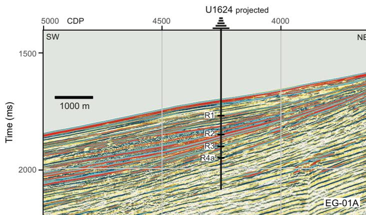
**Figure F16.** Seismic Line EG-01A showing projected location of Site U1624, evident mass gravity deposits associated with past shelf edge glaciations, interpreted reflectors (R1–R4a), and maximum penetration depth to 258 mbsf.
