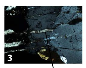
sphene-albite-actinolite veins cutting ilmenite and plagioclase, and earlier fluid inclusion trails
