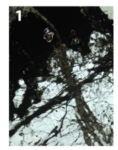
hornblende vein cutting ilmenite (+ rutile) and cut by actinolite
