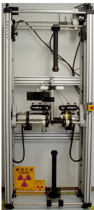
Figure 2-3. A vertical moving sensor MSCL installed in a laboratory in Japan.
