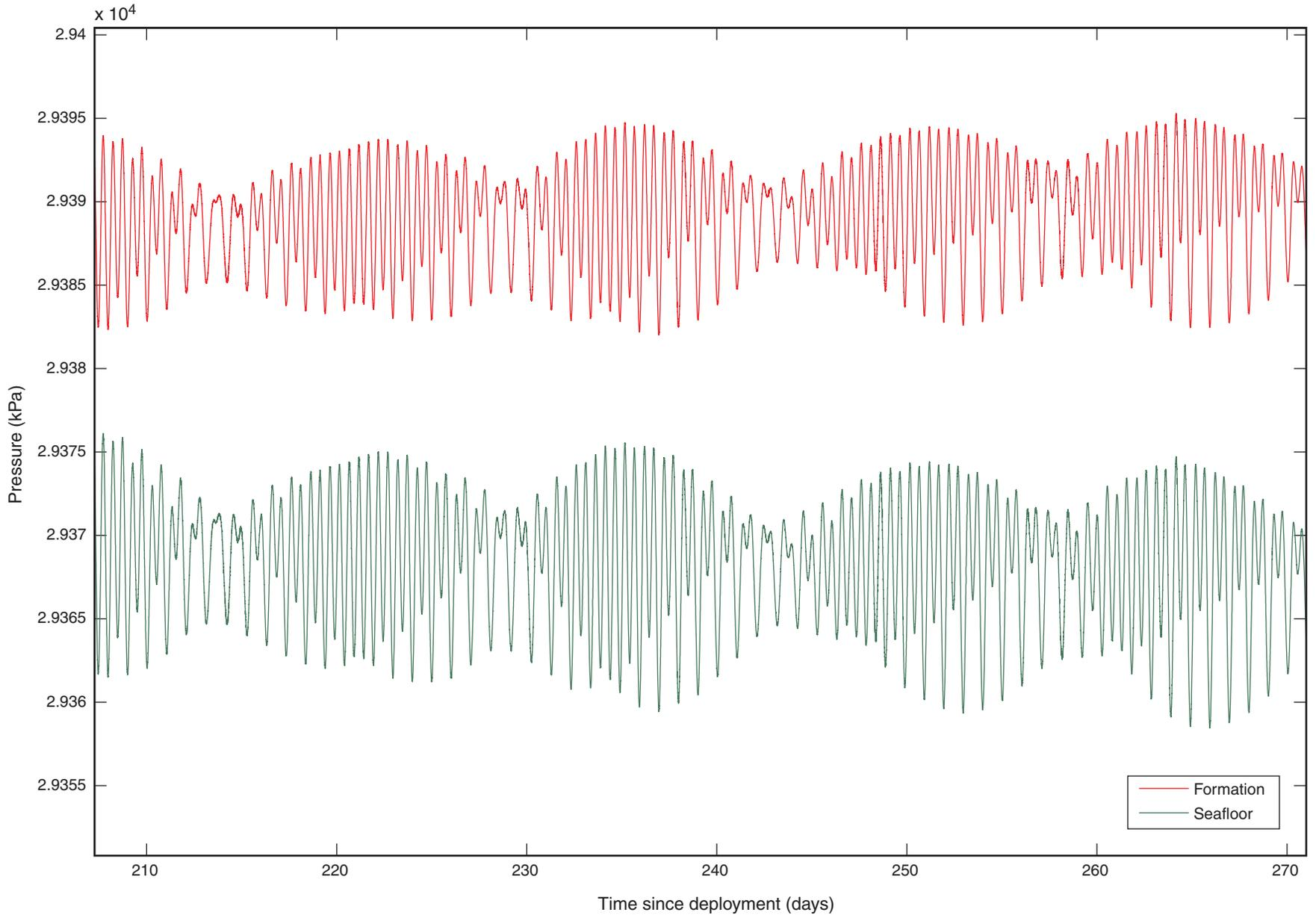
**Figure F9.** Both sensors register a high-frequency response  $\sim 1$  h after Chile M 8.8 earthquake (EQ) on 27 February 2010 and an additional anomaly correlated with the arrival of the tsunami wave (23.5 h later), Site C0010.
