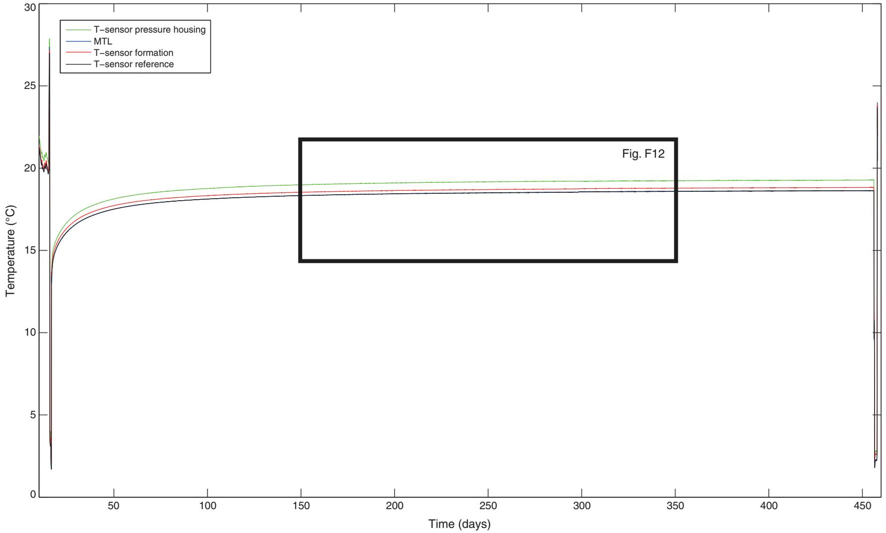
**Figure F12.** Example of temperature perturbations in late May 2010, Site C0010. It remains unresolved why three thermistors show a systematic increase by  $\sim 0.03^\circ\text{C}$ , whereas one drops gently at the same time. MTL = miniature temperature logger.
