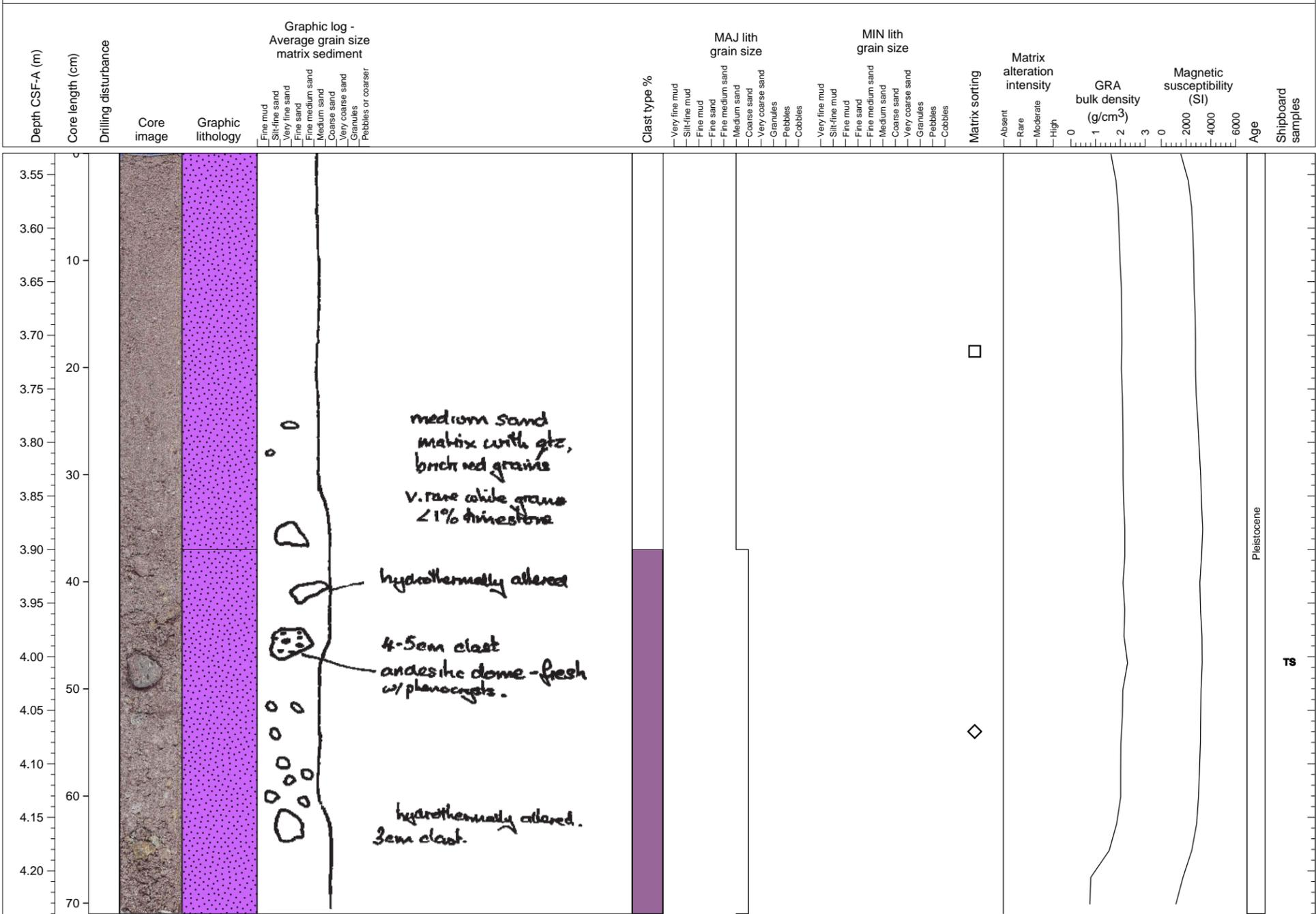
Loose clasts that may not be in place. Mainly andesitic, some oxidized. size to 5 cm.
