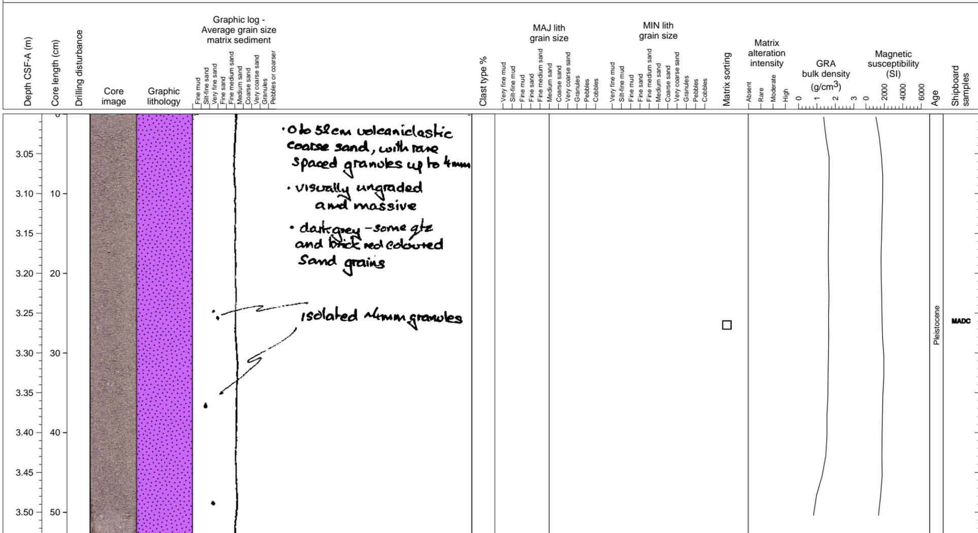
Dark volcanoclastic coarse sand, with clasts up to 4.5 cm in lower part. Clasts mainly andesitic, some hydrothermally altered.
