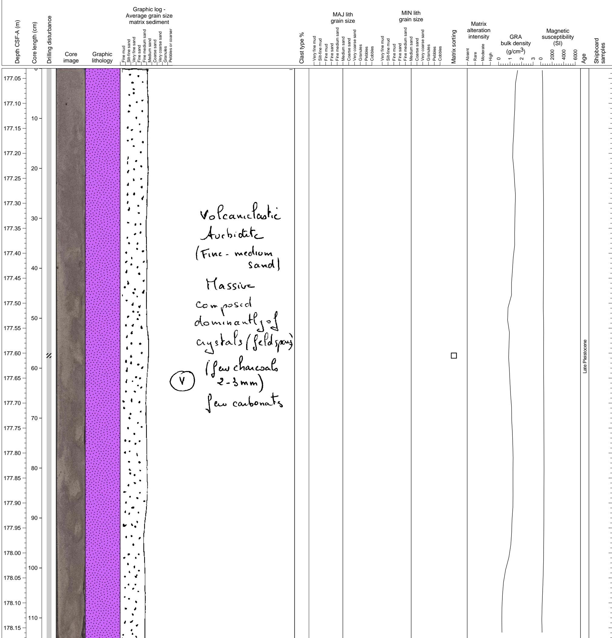
Mixed volcaniclastic-carbonate turbidite sand. Massive, no grading.
