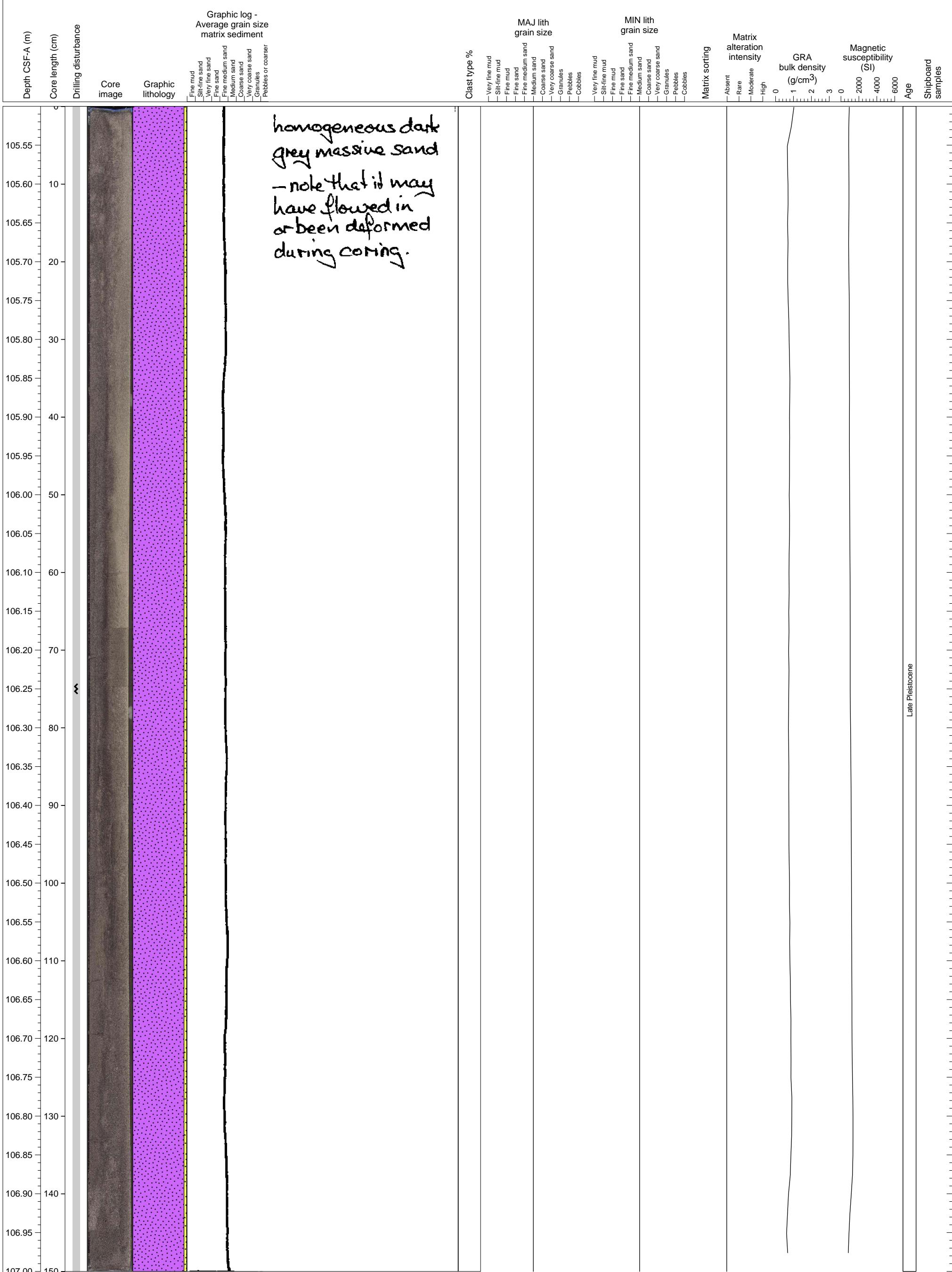
Homogeneous dark grey medium sand with occasional carbonate grains. Massive and may have flowed during coring.
