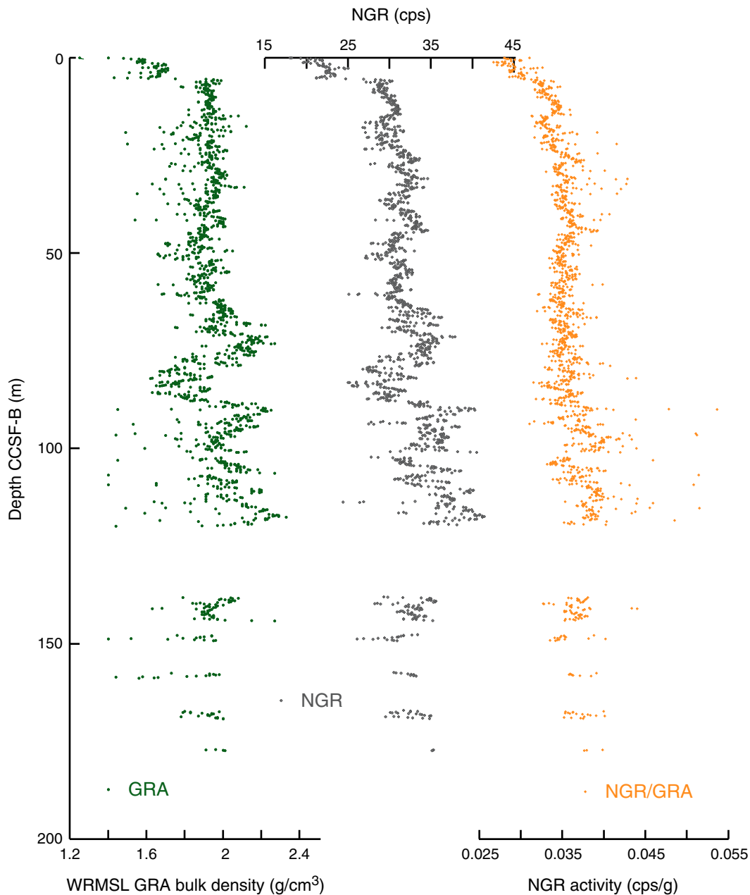
Figure F56. Whole-Round Multisensor Logger (WRMSL) gamma ray attenuation (GRA) bulk density compared to natural gamma radiation (NGR) data, Site U1419. Both data sets are shown after Gaussian smoothing with a 50 cm window and interpolation to constant resolution at 10 cm. NGR is also shown corrected for variability in recovered sediment volume by normalizing to WRMSL GRA bulk density. From 0 to 90 m CCSF-B, data follow the stratigraphic splice; at greater depths, data from Hole U1419A, U1419C, and U1419D cores are combined. In this lower interval, when depth horizons were recovered in multiple holes we use an average of all available interpolated data.
