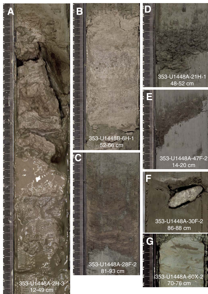
Figure F9. Line-scan images of minor lithologies, Site U1448. A. Volcanic ash likely associated with the Toba eruption, Subunit Ia. B. Light gray volcanic ash, Subunit Ia. C. Pinkish gray volcanic ash, Unit II. D. Thin turbidite composed of black to dark gray bioclastic silt with foraminifers, Unit II. E. Very thin turbidite composed of greenish black bioclastic sand with silt, Unit II. F. Pyrite nodule, Unit II. G. Microfault offsetting mottled brown and greenish gray sediments, Unit IV.
