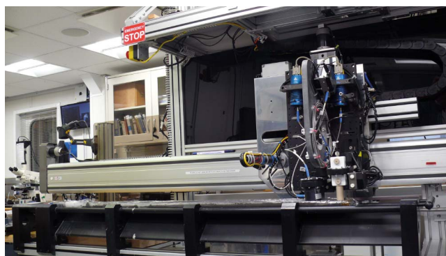
Figure F17. SHMSL for measurements of color reflectance and point magnetic susceptibility on archive section halves.
