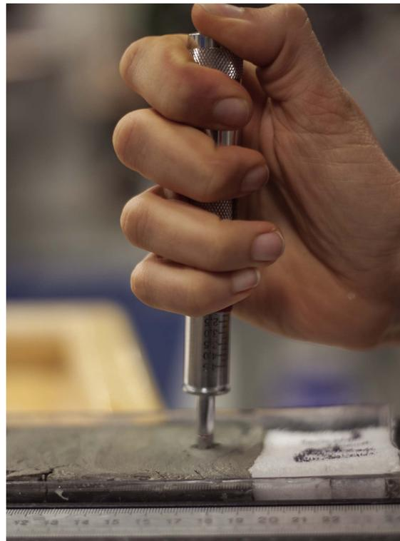
Undrained shear strength can be expressed in terms of total stress in the case of fully saturated materials of low permeability (e.g., clays), denoted by  $S_u$ . The most common strength tests in ship-board laboratories are the vane shear and penetrometer tests, which provide measurement of undrained shear strength ( $S_u$ ) (Blum, 1997). Both tests were used during Expedition 355.
