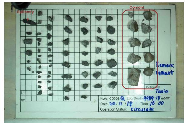
Residues of a 400-cc cuttings sample after washed with 4-mm mesh sieve. Blocky grains in the right side are cement fragments. A splintery caving (upper left) is contained.
