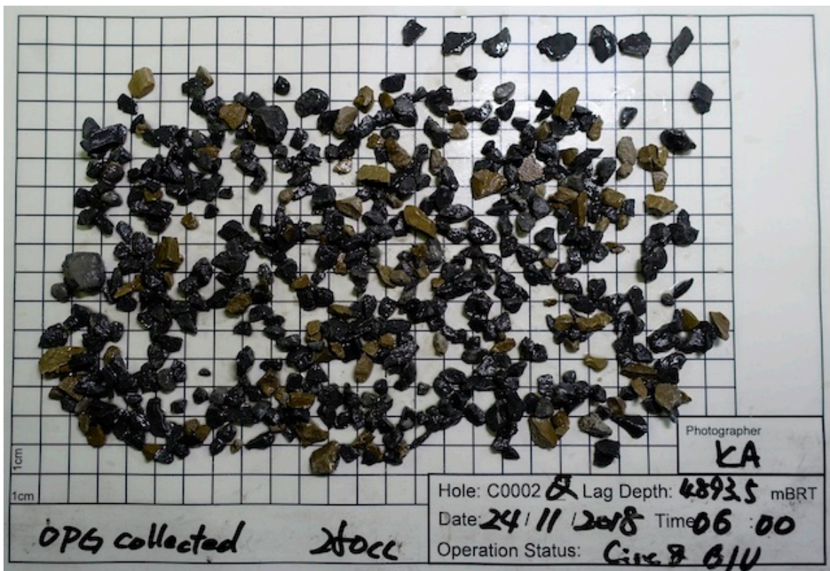
Residues of a 250-cc cuttings sample after washed with 4-mm mesh sieve. Brownish gray grains are cement fragments.
