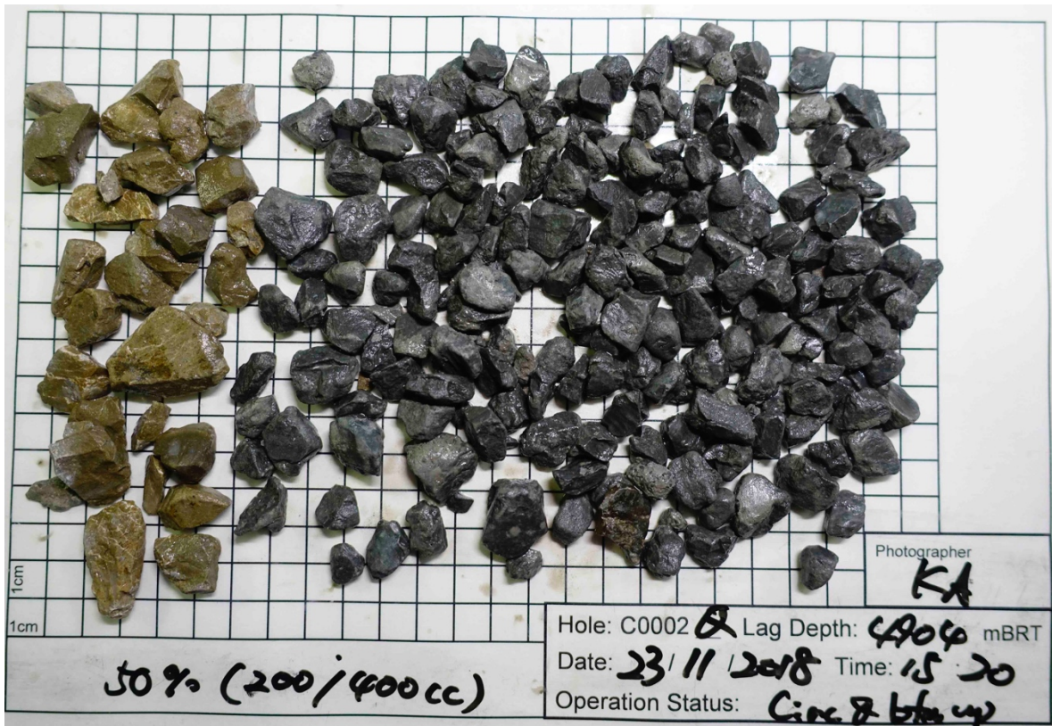
Residues of a 400-cc cuttings sample after washed with 4-mm mesh sieve. Brownish gray blocky grains in the left side are cement fragments.
