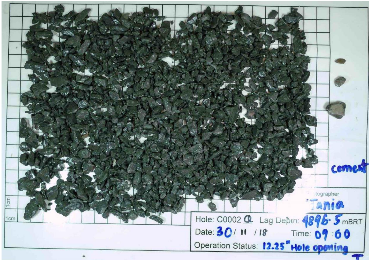
Residues of a 400-cc cuttings sample after washed with 4-mm mesh sieve. Brownish gray blocky grains in the right side are cement fragments.
