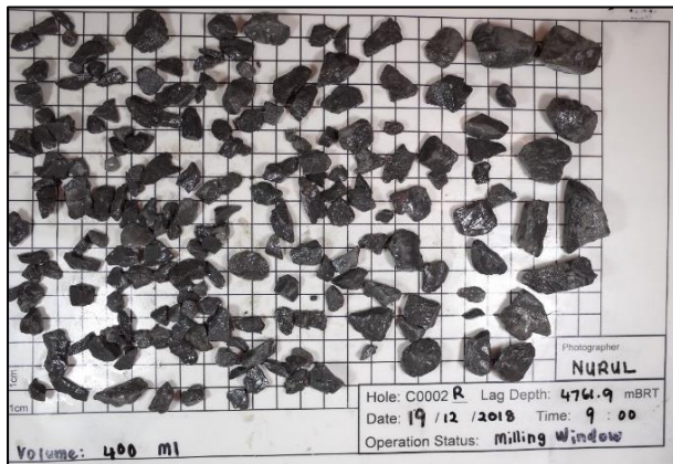
Figure 4 Cuttings and cavings from milling out section #0 rathole on C2R
