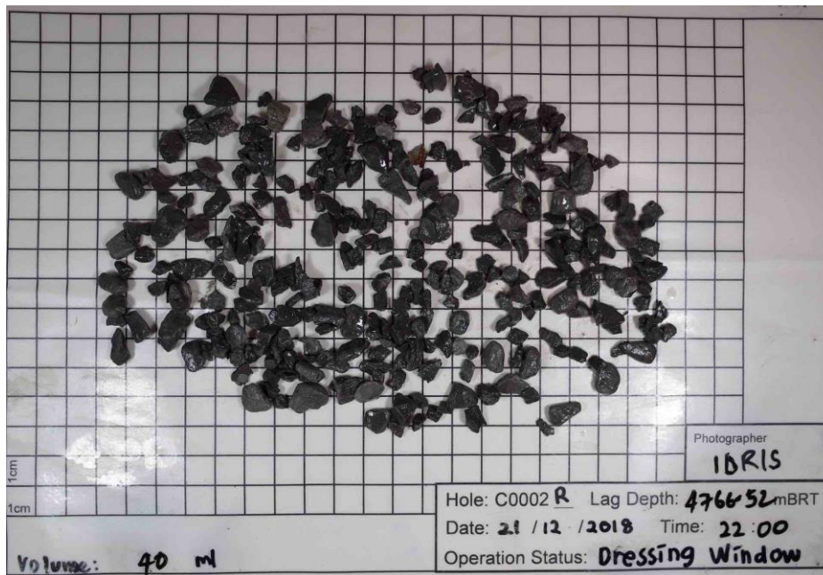
Figure 3 Example of cuttings/cavings \gt \phi 4\text{mm} (taken from 400cc RTG Samples).
