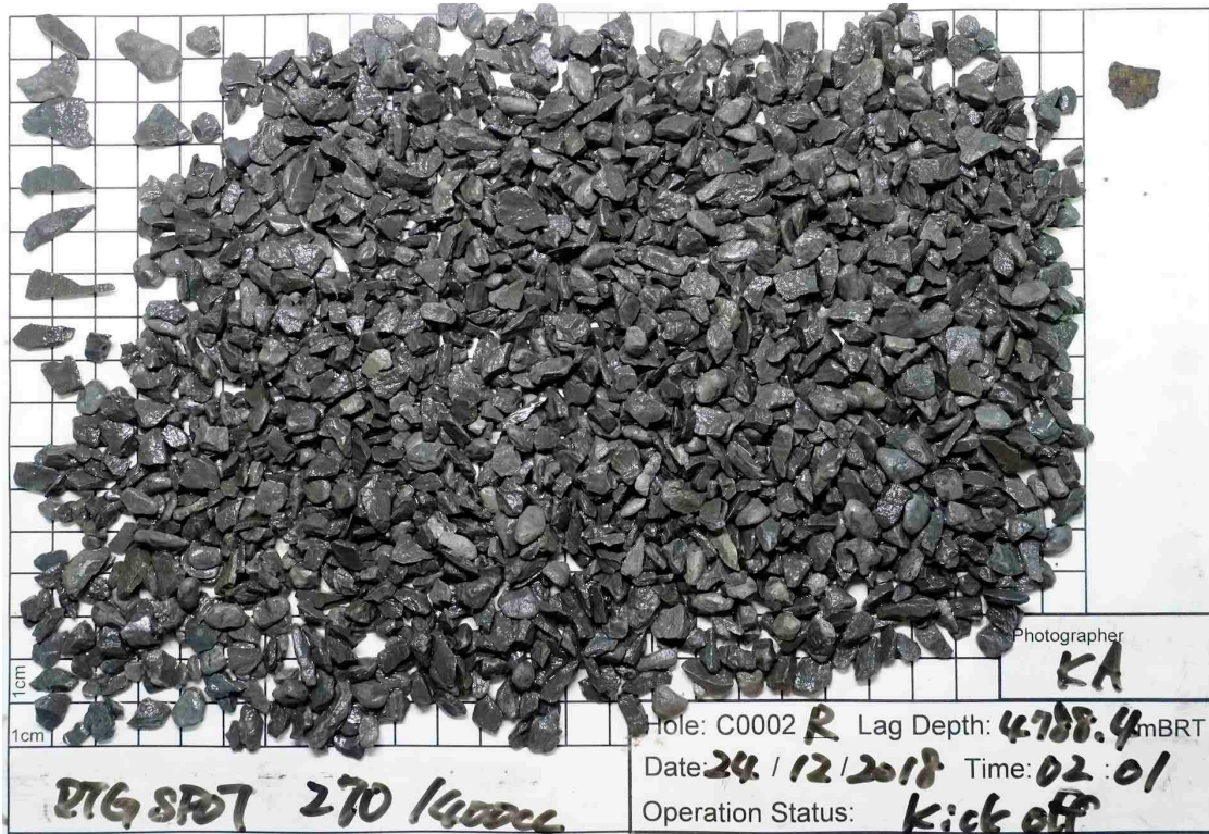
Figure 4: Example of cuttings/cavings > \varnothing 4mm (taken from 400cc RTG Samples).
