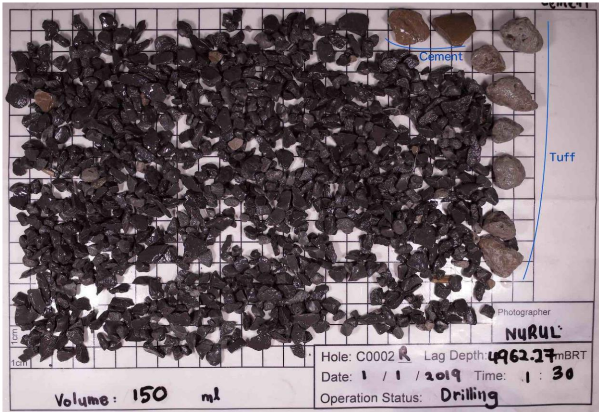
Figure 4: Example of cuttings/cavings > \varnothing 4mm (taken from 400cc RTG Samples). Rounded shale fragments \leq \varnothing 10 mm dominants. Light gray rounded to sub-rounded grains are tuff fragments, probably formed as fresh blocky cavings and with edges worn-down either by up-down circulating in the hole during pumps on/off periods and also further erosion while being transported to the surface.
