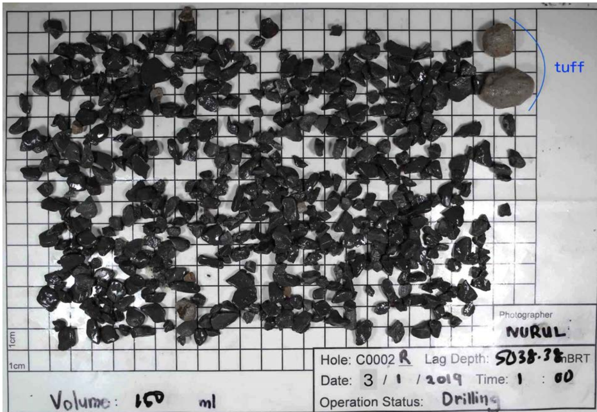
Figure 4: Example of cuttings/cavings > \varnothing 4mm (taken from 400cc RTG Samples). This sample is predominantly rounded shale fragments \leq \varnothing 10 mm, associated with rounded large blocky tuff cavings.
