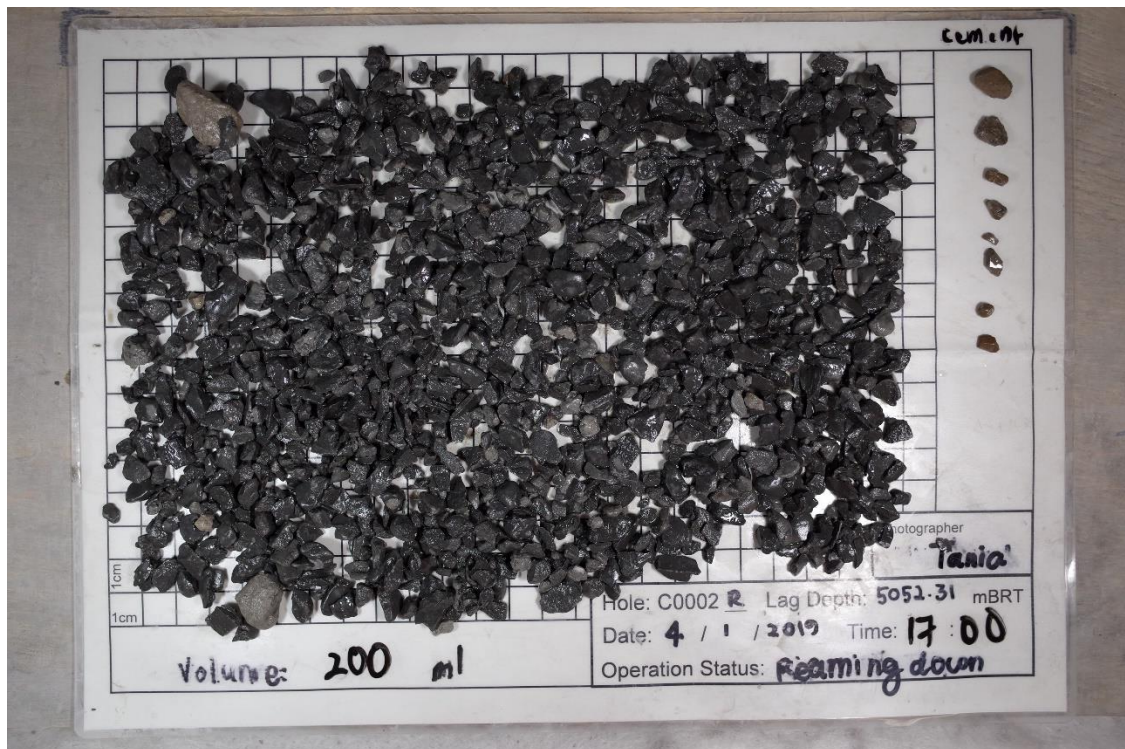
Figure 4 Example of cuttings/cavings > \varnothing 4mm (taken from 400cc RTG Samples). The predominant cuttings are fresh shale fragments \leq \varnothing 10 mm, with trace occurrences of large blocky tuff cavings and angular cement fragments.
