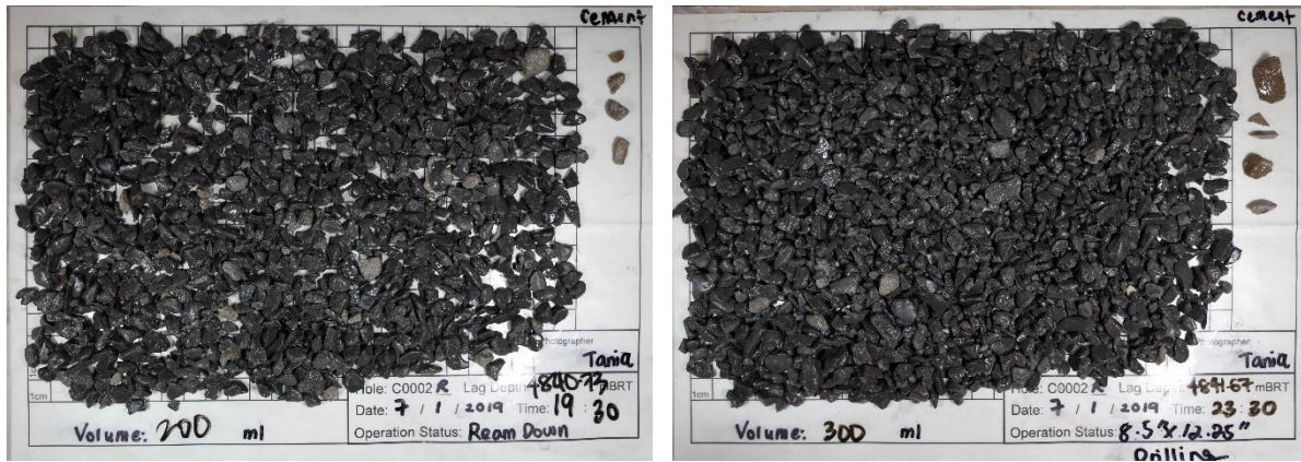
Figure 4 Example of cuttings/cavings > \varnothing 4mm (taken from 400cc RTG Samples). The predominant cuttings above 4,840 mBRT are rounded tuff fragments and below 4,840 mBRT fresh small blocky cuttings \leq \varnothing 10 mm. The cuttings photo at 1930 hrs (left) indicates an abundance of cuttings, but this abundance increases again, as indicated in the cuttings photo at 2330 hrs (right).
