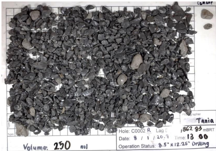
Figure 4 Example of cuttings/cavings > \phi 4mm (taken from 400cc RTG Samples).
