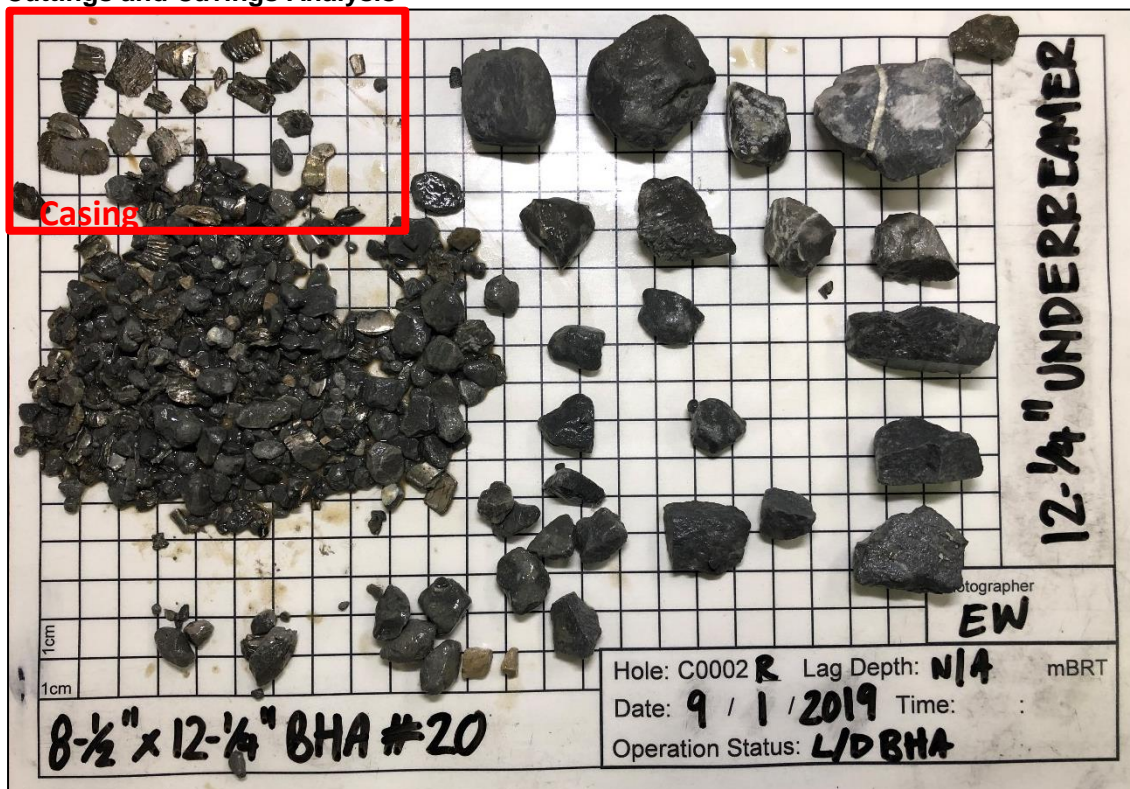
Figure 1 Sample from BHA #20 12-1/4" Underreamer
