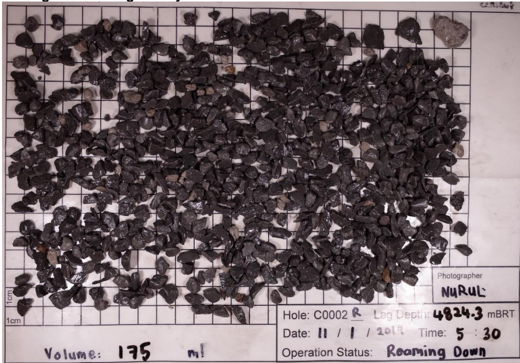
Figure 2 Example of cuttings/cavings > \phi 4mm (taken from 400cc RTG Samples)
