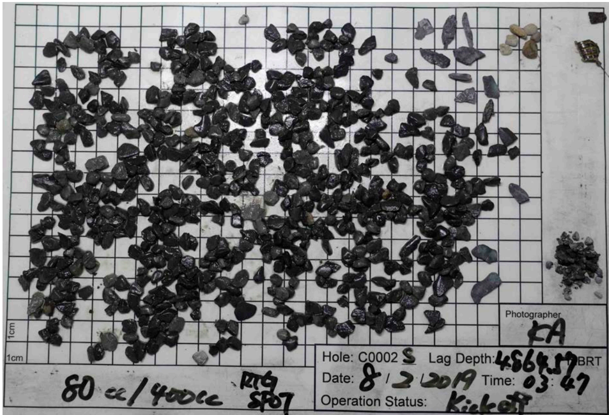
Figure 4 Example of cuttings/cavings > ø 4mm (taken from 400cc RTG Samples).
