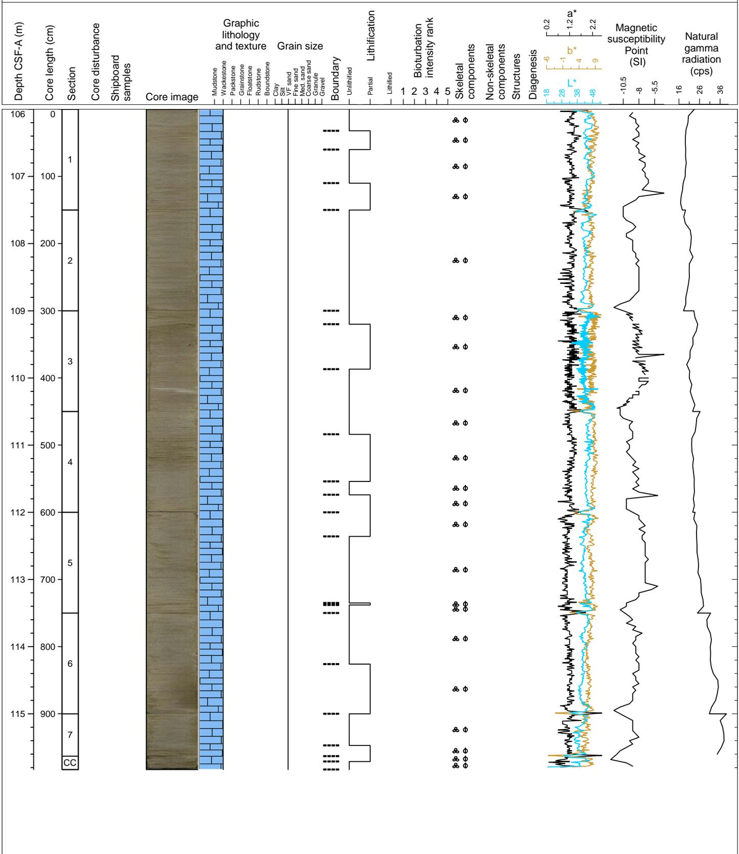
Hole 359-U1467D Core 14H, Interval 115.5-125.3 m (CSF-A)
