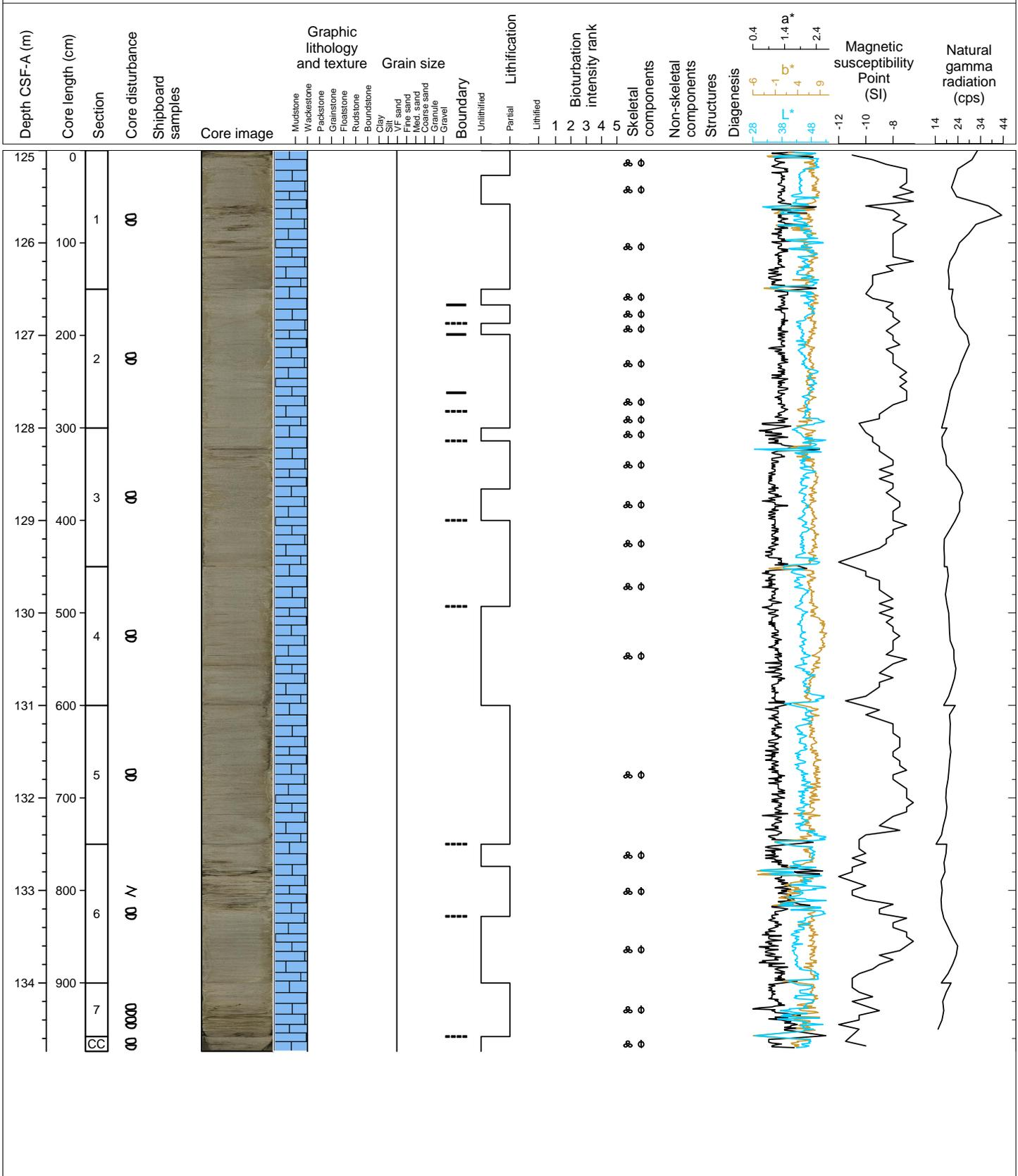
Hole 359-U1467D Core 16H, Interval 134.5-144.17 m (CSF-A)
