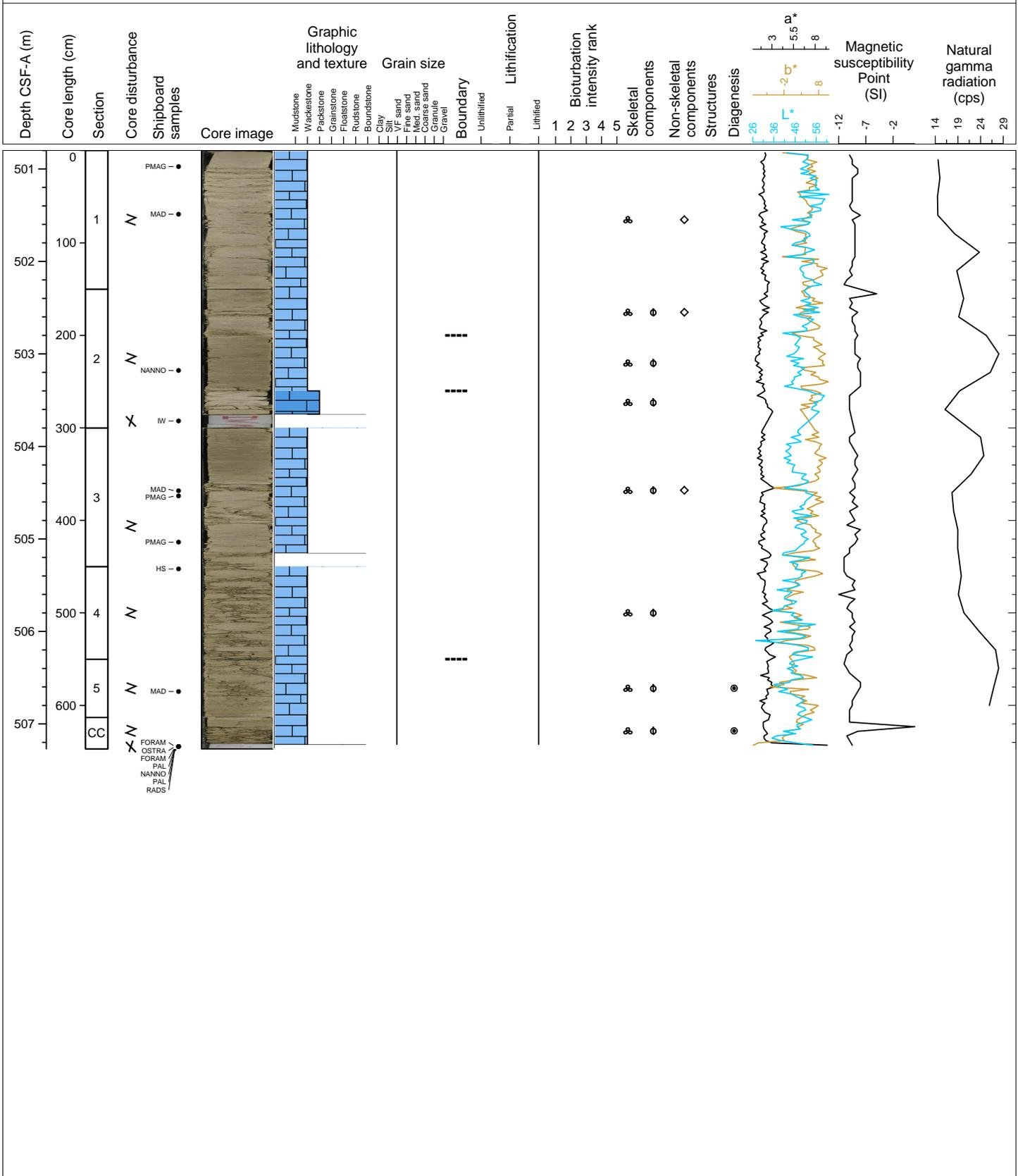
Hole 359-U1467B Core 67X, Interval 510.5-516.71 m (CSF-A)
