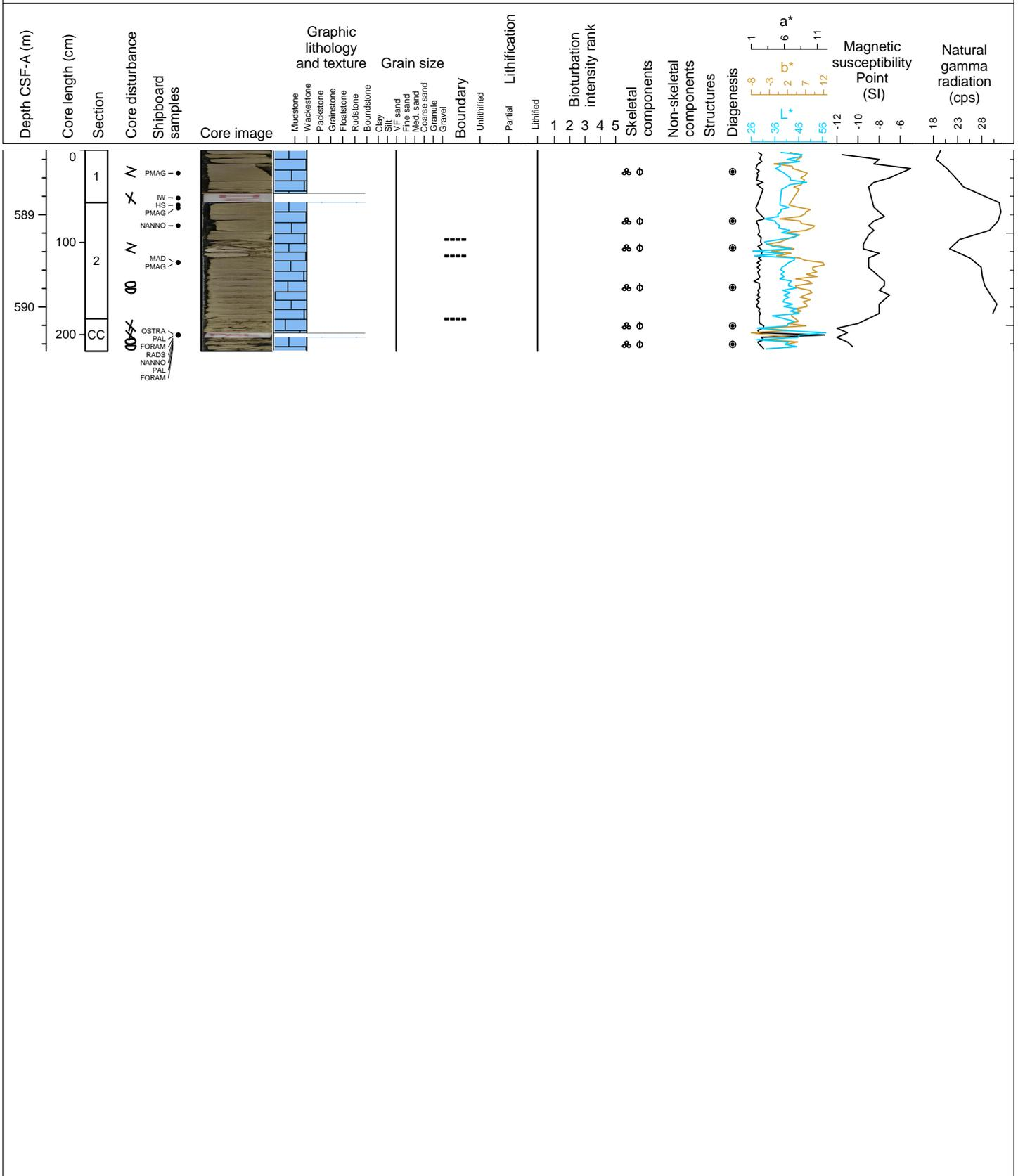
Hole 359-U1467C Core 26X, Interval 598.0-602.64 m (CSF-A)
