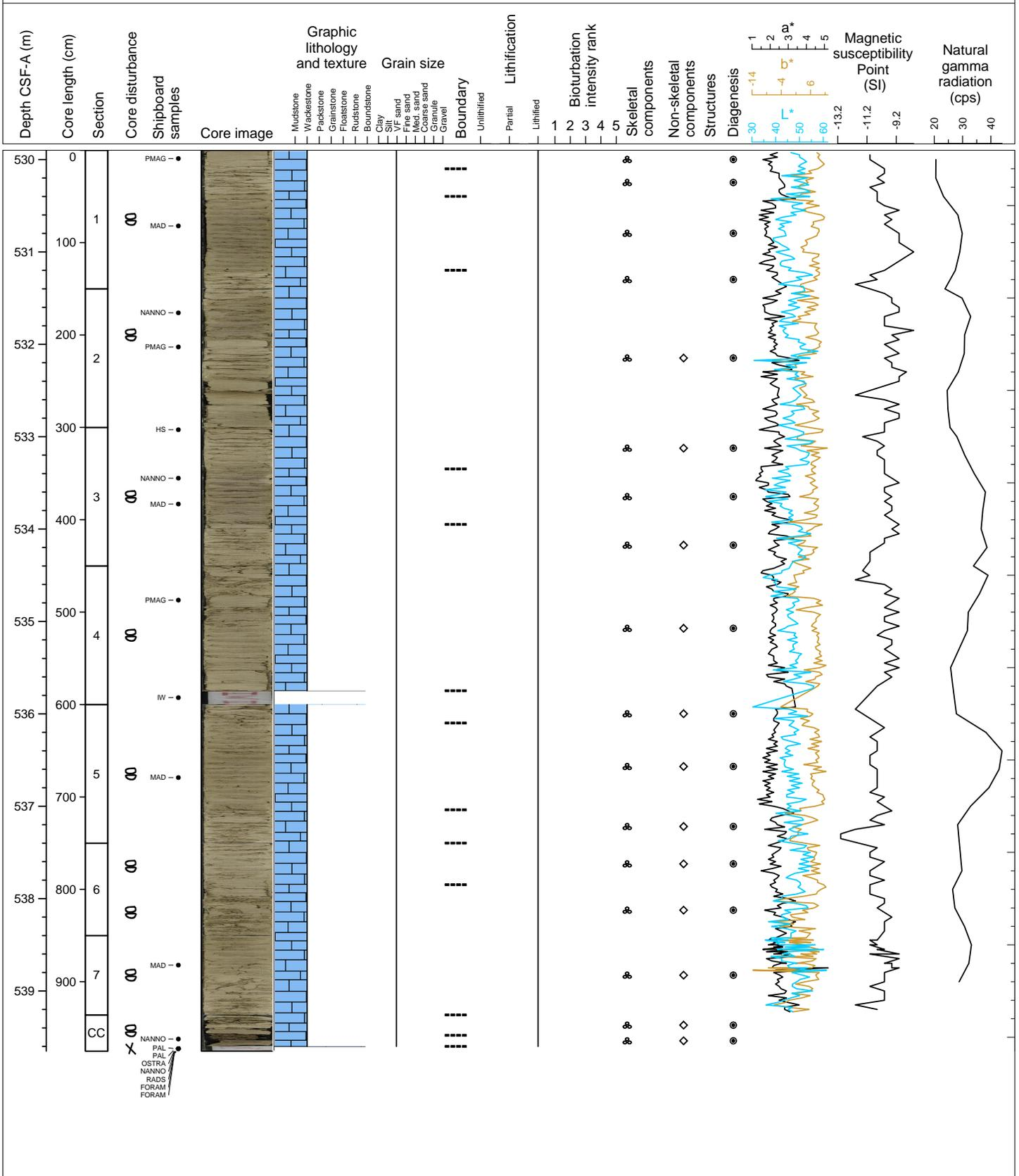
Hole 359-U1467B Core 70X, Interval 539.6-542.07 m (CSF-A)
