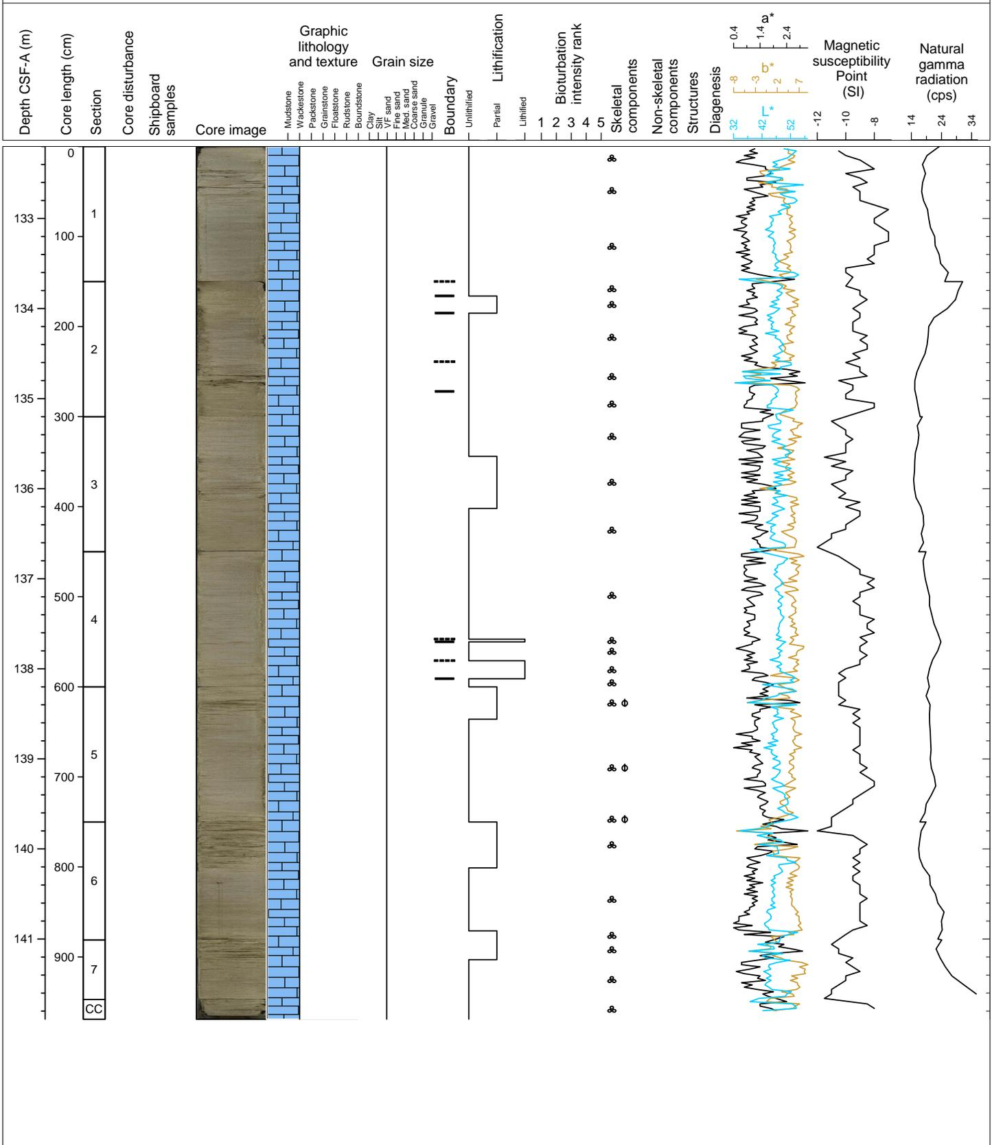
Hole 359-U1467C Core 17H, Interval 141.7-151.62 m (CSF-A)
