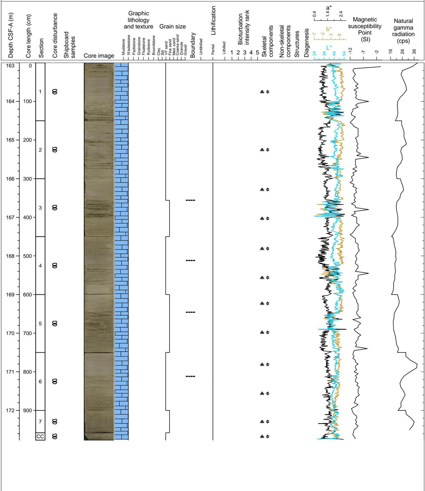
Hole 359-U1467D Core 20H, Interval 172.5-182.36 m (CSF-A)
