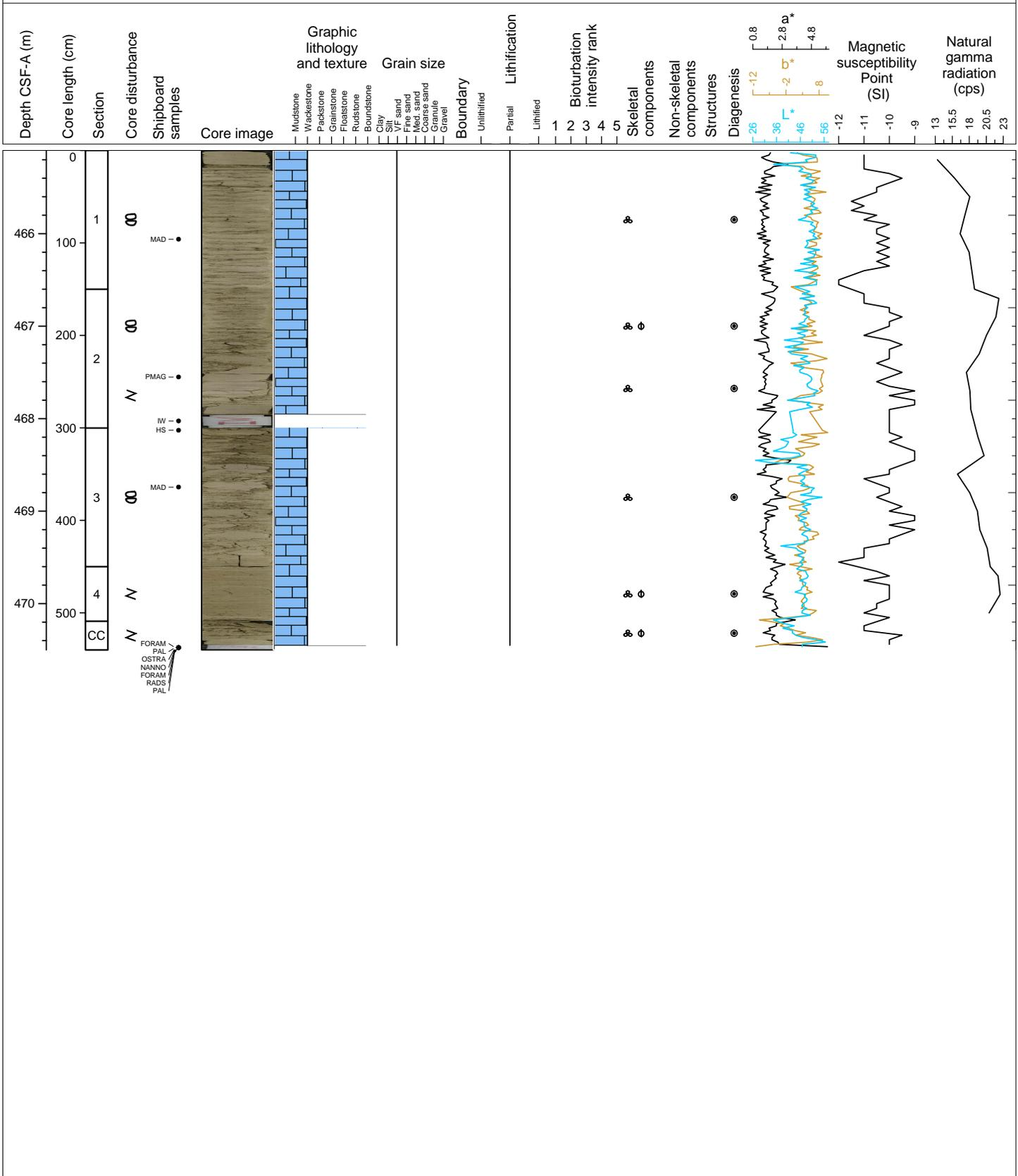
Hole 359-U1467B Core 63X, Interval 471.6-479.62 m (CSF-A)
