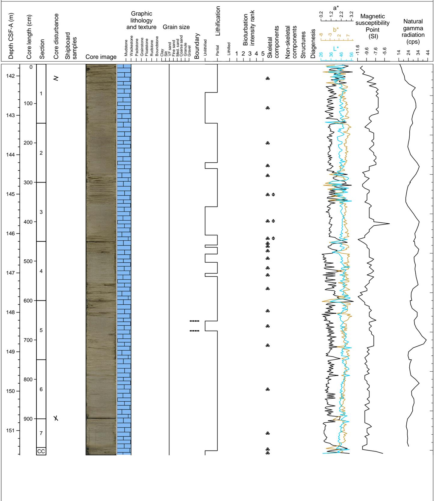
Hole 359-U1467C Core 18H, Interval 151.2-160.99 m (CSF-A)
