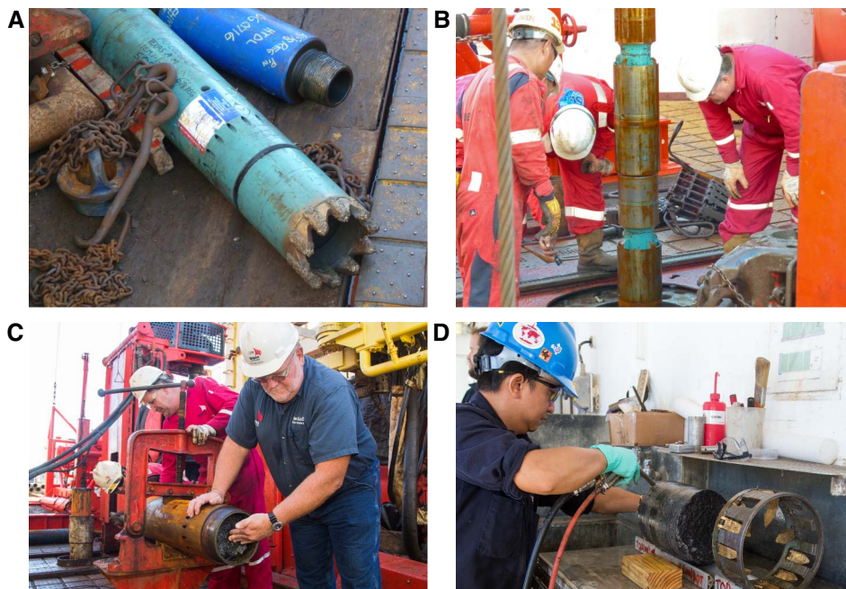
Figure F7. A–B. Hole U1473A BHA Run 13 (fourth RCJB deployment) recovered one of the four lost roller cones.
