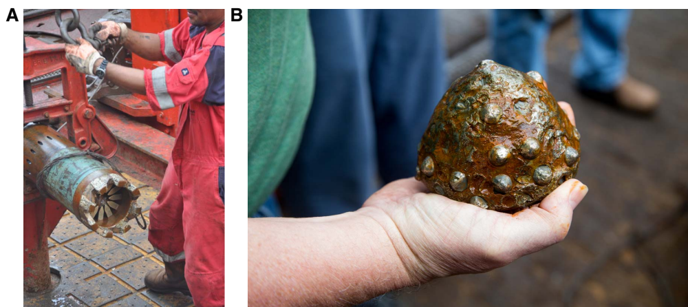
Figure F7. A–B. Hole U1473A BHA Run 13 (fourth RCJB deployment) recovered one of the four lost roller cones.
