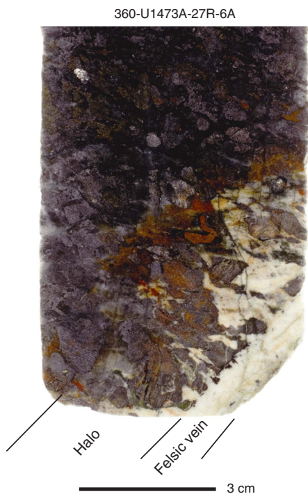
Figure F40. Felsic patch in gabbro, Hole U1473A. Felsic veins seem to infiltrate into the preexisting gabbro (red broken arrows).
