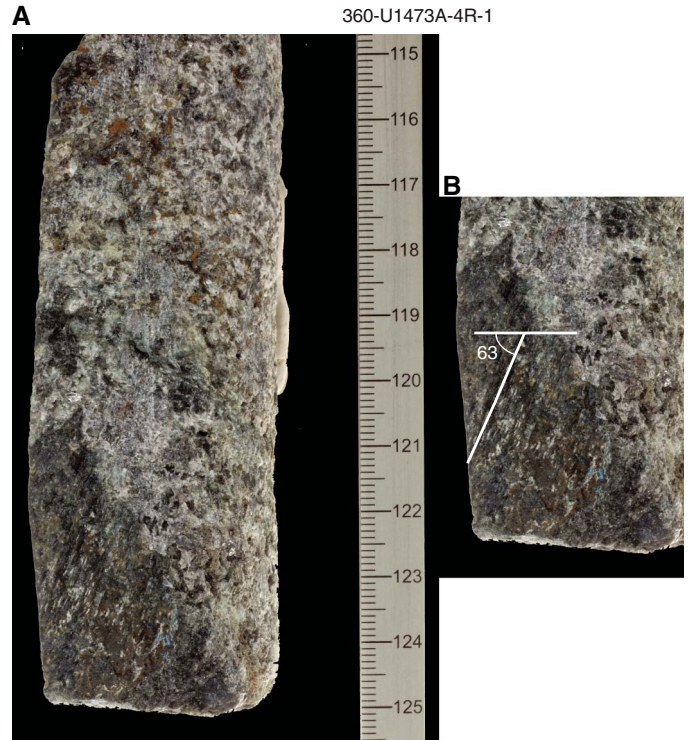
Figure F137. A. Fracture surface with slickenlines on olivine gabbro. B. Annotated image of the slickenlines with rake of 63° from \gamma in the CRF.
