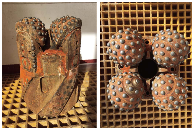
Figure F4. Rotary coring bit used during bit Run 5 to cut lowermost 19.2 m of gabbro in Hole U1473A shows no sign of wear or damage.
