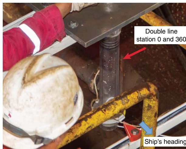
Figure F38. APC assembly used for orientation tool testing, where the working-half double lines were aligned with a pointer that was pointing to the ship's heading.
