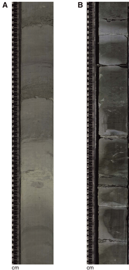
Figure F28. A. Core rated intermediate and ductile in strength. Upward-arching bedding is slight and sediments are more lithified based on use of hammer and chisel to obtain samples (Section U1480F-16F-1). B. Core rated intermediate and brittle in strength. Drilling-induced biscuiting with associated gouge was occasionally observed (Section U1480F-92X-1).
