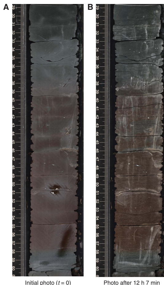
Figure F17. Core image scanned (A) soon after core splitting and (B) ~12 h later (U1481A-32R-6, 29–61 cm; 1438.45–1438.77 mbsf). Note that existing fractures have become wider and new fractures have formed. Entire 30 cm long interval is within a single drilling biscuit.
