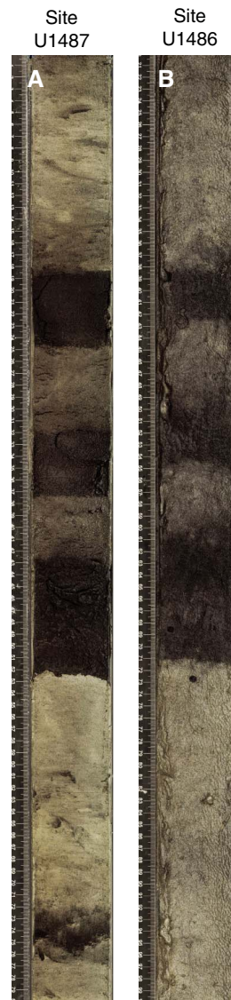
Figure F12. Tephra layers produced by the same volcanic event identified at (A) Site U1487 (U1487A-9H-1A, 18–53 cm) and (B) Site U1486 (U1486D-15H-3A, 38–71 cm).
