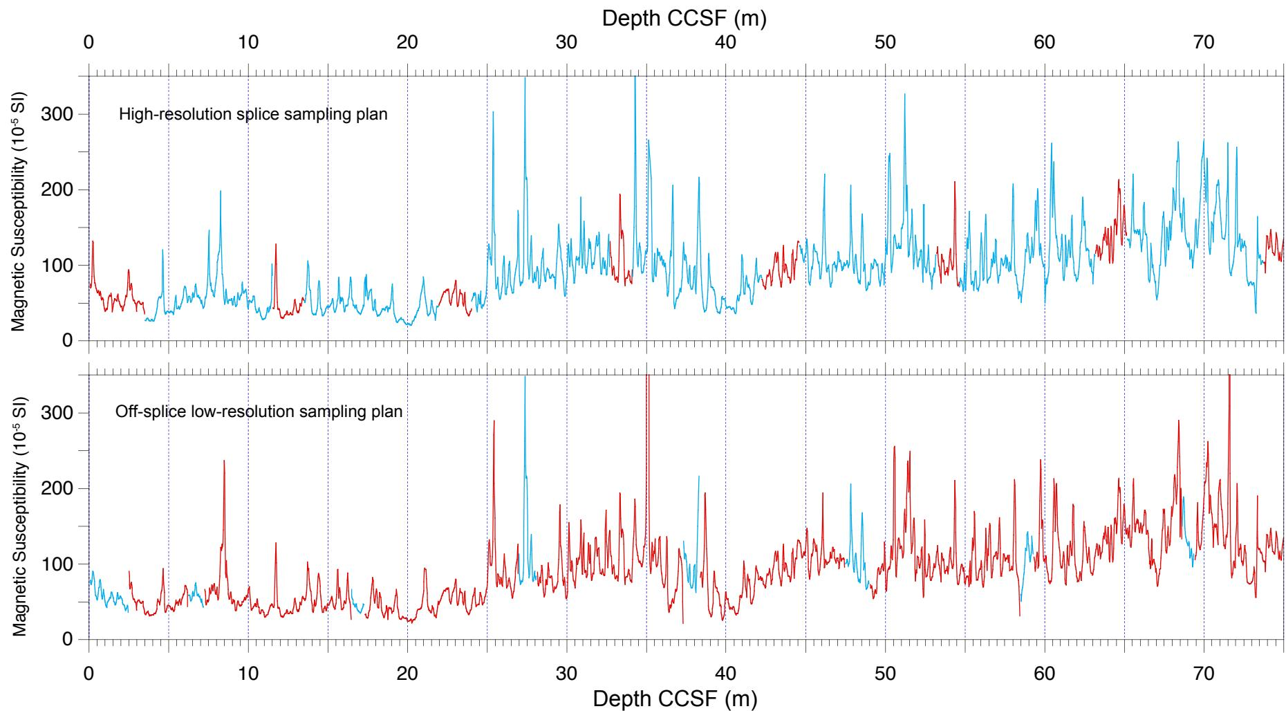
Supplementary Figure 6A–B. Comparison of magnetic susceptibility records at Site U1487 constructed using the high-resolution splice interval table (top panel) and the off-splice interval table for low-resolution sampling (bottom panel).
