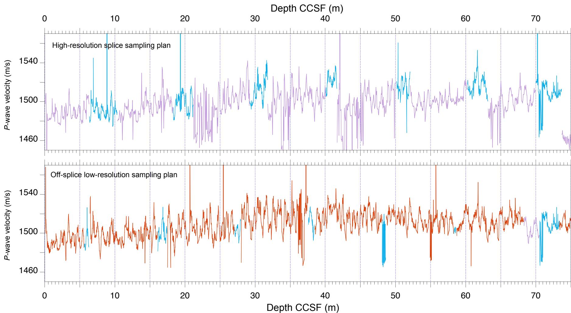
Supplementary Figure 7A–E. Comparison of P-wave velocity records at Site U1488 constructed using the high-resolution splice interval table (top panel) and the off-splice interval table for low-resolution sampling (bottom panel).
