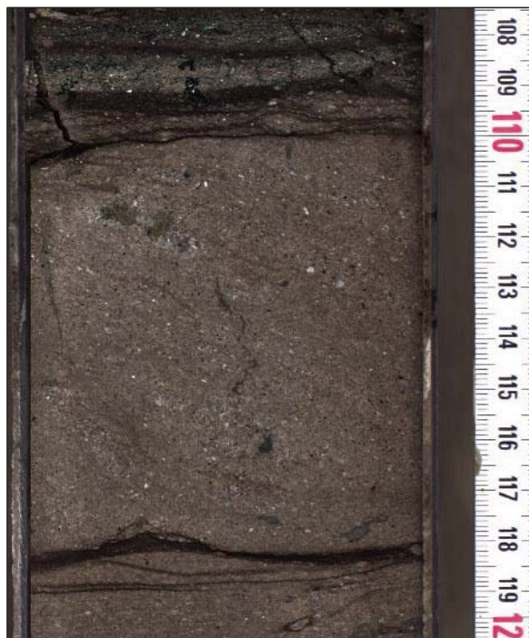
Figure F5. Cross-lamination in suevite at the top of Subunit 2A (364-M0077A-40R-1).
