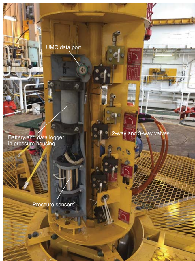
Figure F14. Bay 1 of LTBS head, holding the PSU with four high-precision quartz pressure sensors (Paroscientific, Inc.) and two-way and three-way valves. Note cylindrical pressure housing with data logger and PPC unit. See text.
