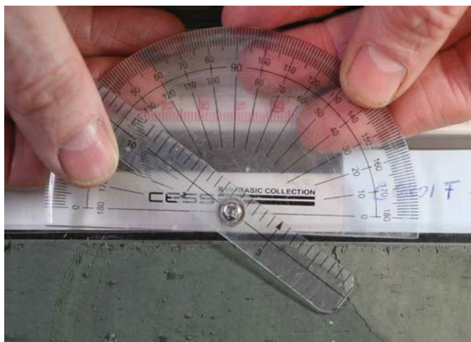
Figure F25. Modified protractor used to measure apparent dip angles, bearings, plunge angles, and rakes of planar and linear features in the working half of split cores.
