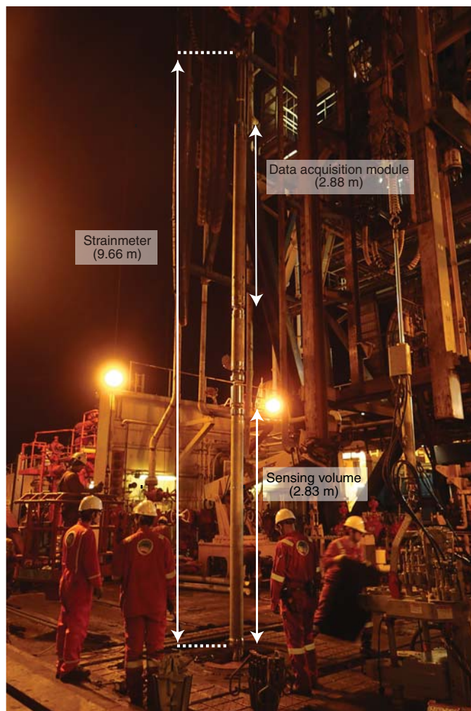
Figure F12. Strainmeter suspended from rig floor, Hole C0010A.
