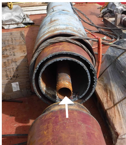
Figure F5. The current mechanical state of Hole 1200C includes a PVC 3 inch schedule 80 pipe with a 3.5 inch OD that is likely sealed with five O-rings in the seal sleeve. This PVC has a maximum ID of 2.5 inches (63.5 mm) at the coupling. The seal sleeve rises from the latch and has a 5.25 inch OD with a 3.500 to 3.505 inch ID seal surface. The threaded end of the CORK upper mandrel, which screws into the seal sleeve, remains in the seal sleeve where the CORK parted. The upper mandrel has a 4 inch ID and a 4.5 inch OD.
