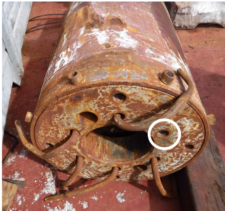
Figure F1. Base of the recovered portion of the CORK body, including five of six latching rods, Hole 1200C. The circle highlights the missing rod. Bending of the rods was exacerbated upon recovery when the CORK was set down on the deck.
