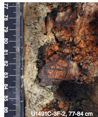
Figure F9. Ultramafic clast exhibiting red weathering with a black (Mn-rich?) crust (366-U1491C-3F-2, 77–84 cm).
