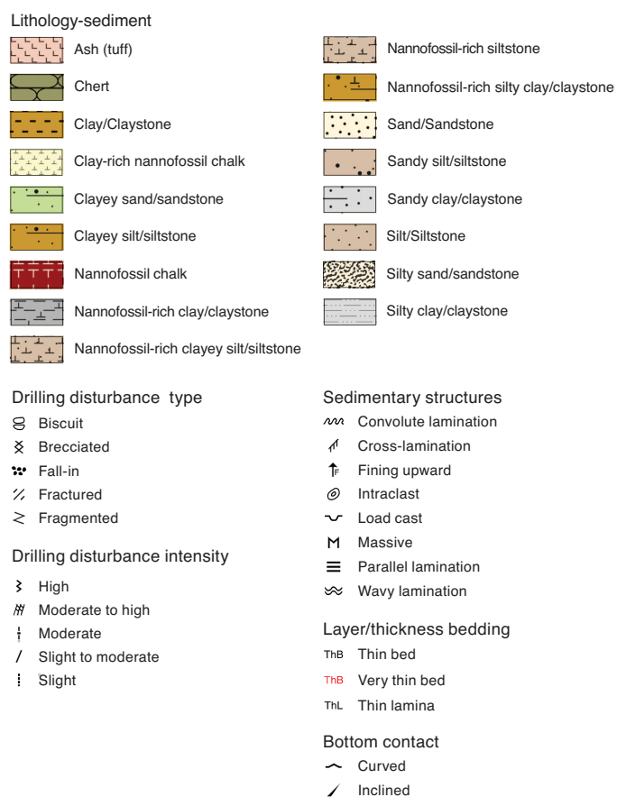
Figure F1. Lithology patterns and symbols used for visual core description of sedimentary intervals, Expedition 368X.
