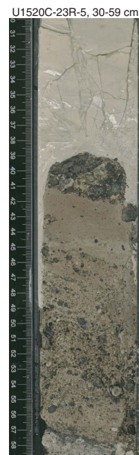
Figure F25. Contact between Unit IV chalk and Unit V volcanoclastic conglomerate at 848.45 mbsf, Hole U1520C. Contact is interpreted to be a significant unconformity.
