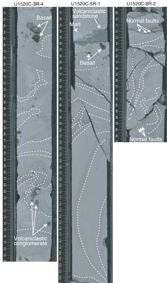
Figure F20. Debris flow deposits in Unit IV showing flow banding in marl, zones of normal faults, and clasts of basalt, volcanoclastic conglomerate, and marl, Hole U1520C. Dashed lines enhance boundaries between contrasting lithologies.
