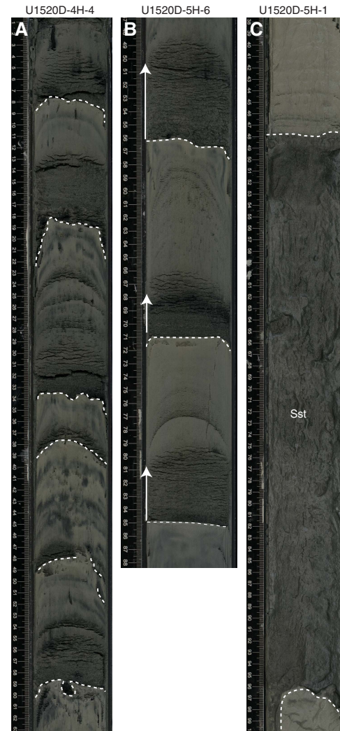
Figure F8. Typical Unit I lithologies, Hole U1520D. A. Thin-bedded silty turbidites. B. Thin- to medium-bedded sandy turbidites showing normal grading (arrows). C. Thick-bedded sandy turbidite. Note that much of the dark staining is due to metastable mackinawite. Sst = sand. Dashed lines = bases of inferred turbidites.
