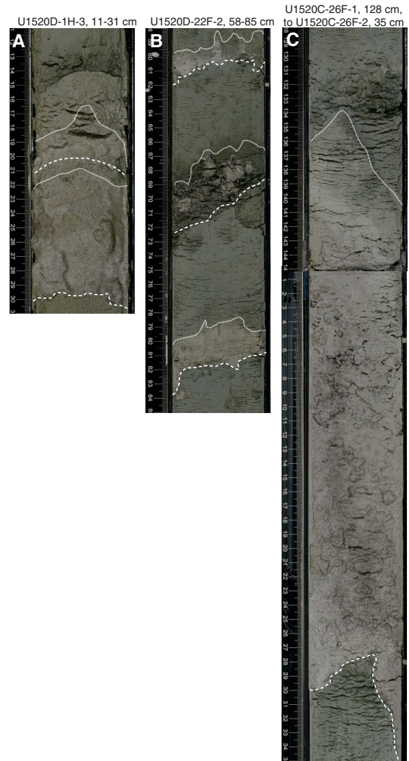
Figure F32. Examples of tephra layers in Units I-III, Holes U1520C and U1520D. Dashed lines = base, dotted lines = presumed top of original ash layers.
