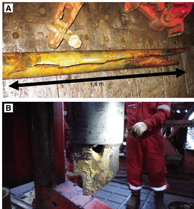
Figure F10. Drill string components damaged from downhole corrosion. A. Parted end of drill pipe (laid out on the rig floor) recovered from Hole U1528D after losing the lowermost ~172 m of drill string including the BHA during drilling operations upon the seventh reentry (Credit: Tobias W. Höfig, IODP). B. Heavily corroded latch sleeve, recovered from the last coring attempt in Hole U1528D, showing native sulfur and sulfate encrustations that resulted from interaction with highly acidic, S-rich fluids rising through the drill string (Credit: Stephen Midgley, IODP).
