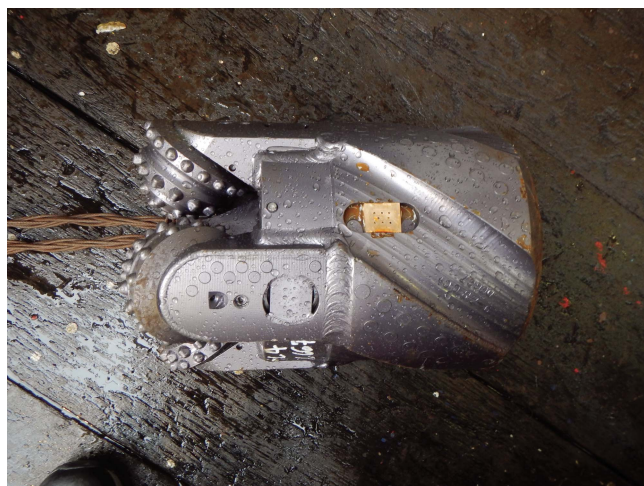
Figure F2. RCB coring bit used during Expedition 376. Bit has inserted perforated brass holder containing fractured quartz crystals designed to trap borehole fluids while implementing coring. (Credit: Tobias W. Höfig and IODP)
