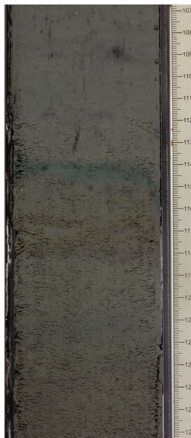
Figure F4. Example of color banding at diatom ooze–silty clay transition, Unit I (382-U1536A-19H-7, 108–124 cm). Green layer contains minor amounts of glauconite.
