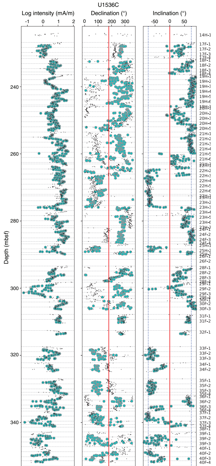
Figure F26. Intensity of remanence, declination, and inclination at 15 mT AF demagnetization level, Hole U1536C. Horizontal dashed lines = section breaks, black dots = original (unedited) data, large cyan dots = edited and adjusted values as described in text, vertical dashed lines in inclination = GAD predicted values for site latitude.
