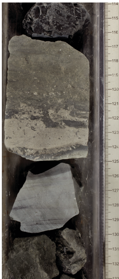
Figure F11. Two drilling biscuits (382-U1536E-32R-1, 117–130 cm). Lower-most biscuit is laminated, quartz-rich mudstone; upper biscuit contains quartz-rich siltstone overlain by finer grained mudstone. Lower portion of upper biscuit is heavily bioturbated.
