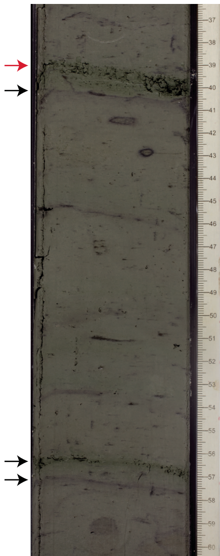
Figure F4. Color banding (black arrows; incipient glauconite formation?) and burrow-rich layer (red arrow) (382-U1537A-7H-5, 37–60 cm).
