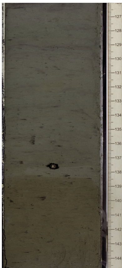
Figure F6. Sharp color boundary between varieties of silty clay (382-U1537A-12H-3, 126–144 cm).
