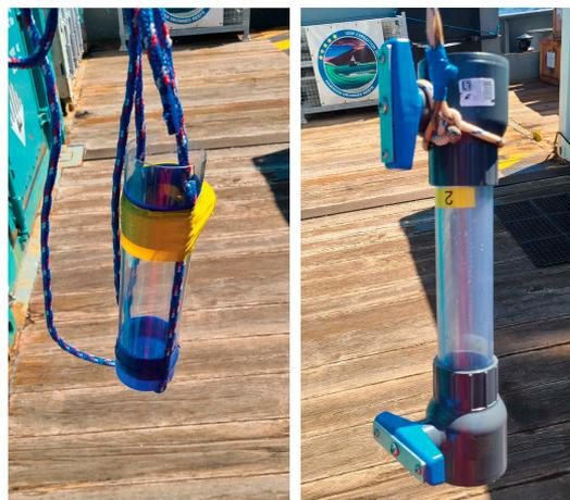
**Figure F22.** SSW sampling devices used during Leg 1 (left) and Leg 2 (right), Expedition 389.
