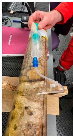
**Figure F21.** IW sampling using a Rhizon sampler connected to a 24 mL all-plastic disposable syringe, Expedition 389.
