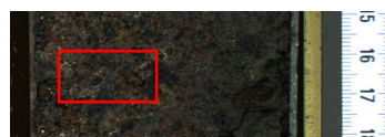
Figure F10. Altered lava rock fragment analyzed using XRD (389-M0096F-4R-1, 15–18 cm) (see Geochemistry). Red box = geochemical sampling location.
