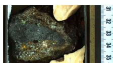
Figure F5. Lithologies, Hole M0096C. Picrobasalt lava clast consisting of a 10%–15% crystallinity interior with round vesicles (389-M0096C-1R-1, 31–35 cm). It has a visually fresh interior and a highly altered (calcium carbonate and Fe oxide replacement) rind.
