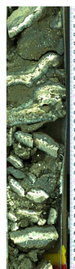
Figure F4. Lithology, Hole M0101A. Coralg-al-microbialite boundstone characterized by laminar corals and thin CCA (7R-1, 20–50 cm).
