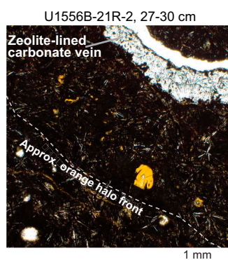
Figure F64. Typical occurrence of bright yellow clay replacing groundmass and filling voids within an orange halo around a zeolite + carbonate vein (PPL), Hole U1556B.
