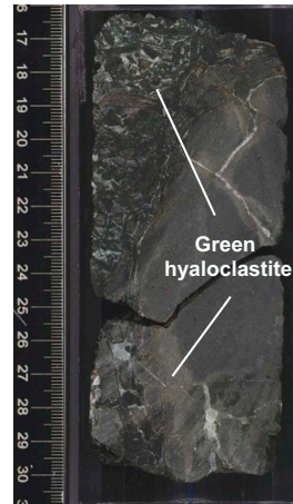
Figure F35. Green hyaloclastite, Subunit 12f (390-U1556B-54R-2 [Piece 2, 16–31 cm]).
