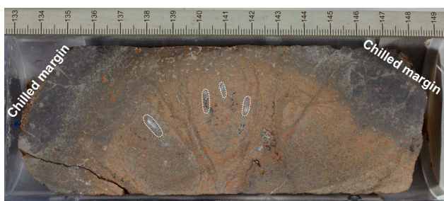
Figure F28. Arcuate chilled pillow margin showing radial fractures and elongation of larger vesicles perpendicular to chilled margin (dotted lines) (390-U1556B-29R-4, 133–149 cm). Notice also paucity of orange spots (i.e., olivine phenocrysts), suggesting this may be a different magma type encountered for the first time in Unit 8.
