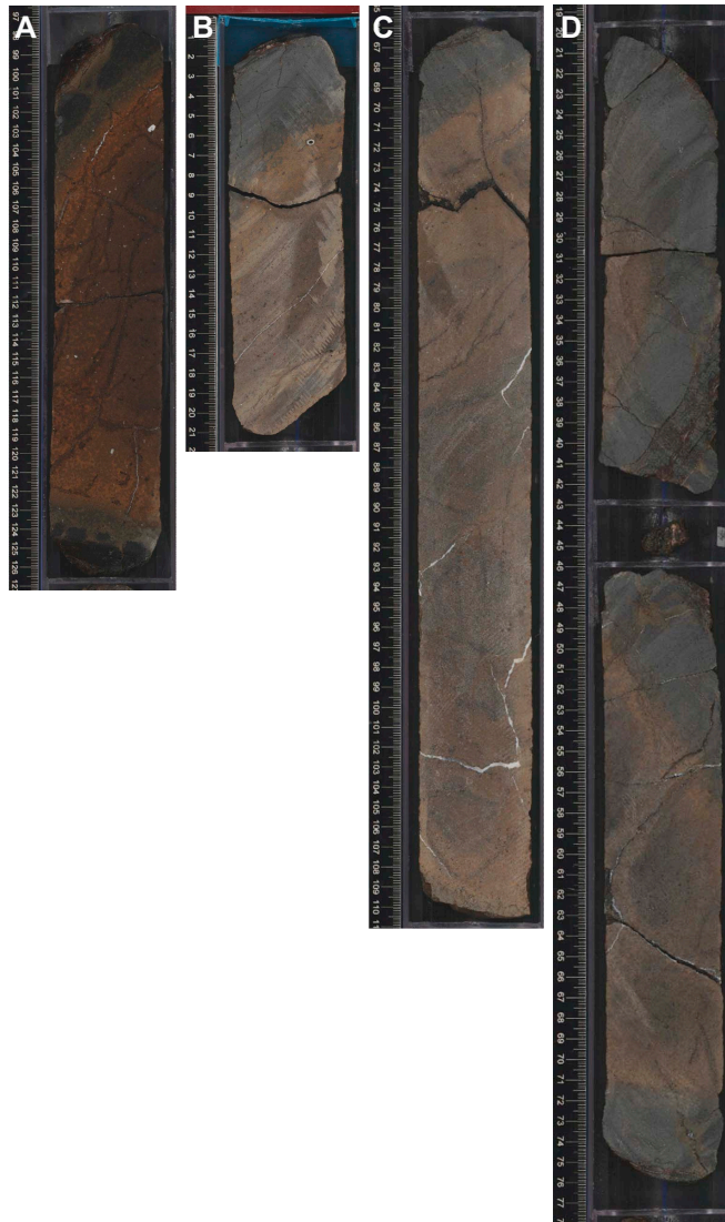
Figure F36. Examples of paired chilled margins in old red pillow lavas, Hole U1556B. A. 40R-1 (Piece 15, 97–126 cm). B. 40R-3 (Piece 1, 0–21 cm). C. 40R-3 (Piece 6, 66–111 cm). D. 44R-2 (Pieces 3–5, 19–78 cm).
