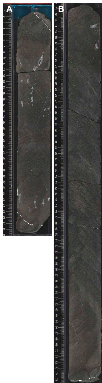
Figure F25. Chilled margins (white dotted outlines), Hole U1556B. A. Chilled margins at high angles to core vertical (20R-6 [Piece 1, 0–39 cm]) showing tendency for large, irregularly shaped vesicles to be concentrated in bands ~4–6 cm away from a chilled margin. B. Horizontal chilled margins of some longer pieces (i.e., thicker flows) (20R-1 [Piece 3, 11–75 cm]).
